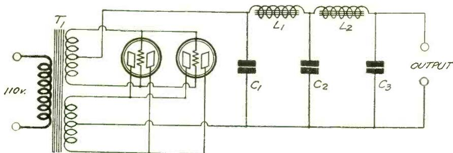
THE CIRCUIT DIAGRAM OF A B BATTERY ELIMINATOR IN WHICH TWO TYPE —80 RECTIFIER TUBES ARE CONNECTED IN PARALLEL TO IMPROVE THE VOLTAGE REGULATION OF THE CIRCUIT. CIRCUIT REQUESTED BY ROGER W. NORTON
