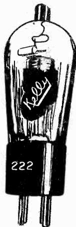
AFTER having tried many screen grid tubes, many specialists have made Kelly 222 their choice. Our 222 stands up! Filament is not critical, but 3.3 volts work best. Plate voltage may be from 90 to 180, but negative bias of 1.5 volts remains the same. The screen grid voltage, G post of socket, may be 22 to 45 volts, depending on how much amplification you want. A working amplification of 60 is easily obtainable (60 mu.).
