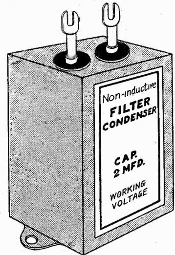
Actual size of new 2 mfd. non-inductive filter condenser for power supplies. 2 1/2" high including lugs, 1 3/16" wide, 1 3/16" front to back. Mounting holes 1 1/2" apart.
