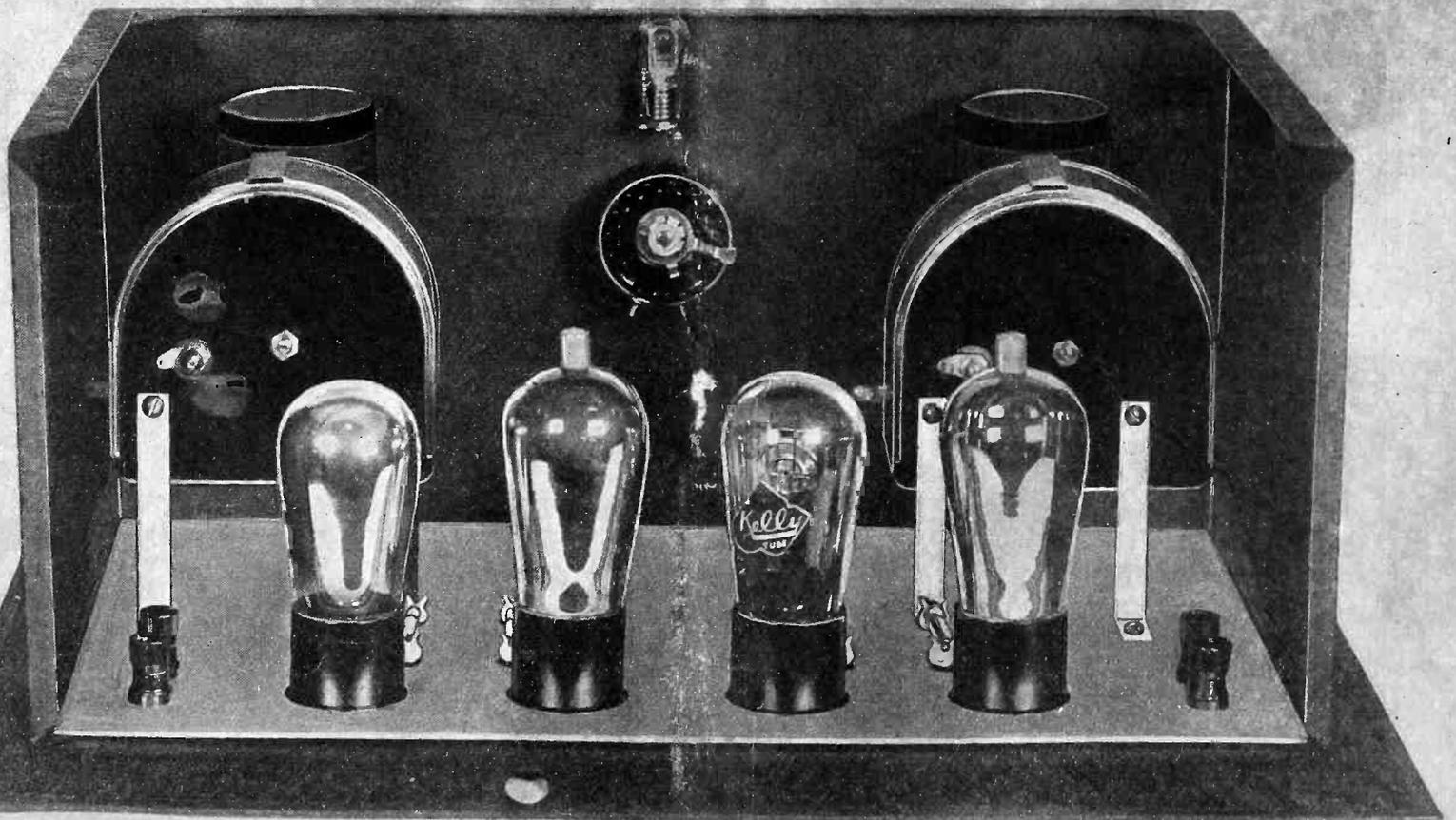
Rear View of Exceptional 4-Tube Set Using Two 222 Tubes, One 240 and One 112A. See pages 3, 4 and 5.
