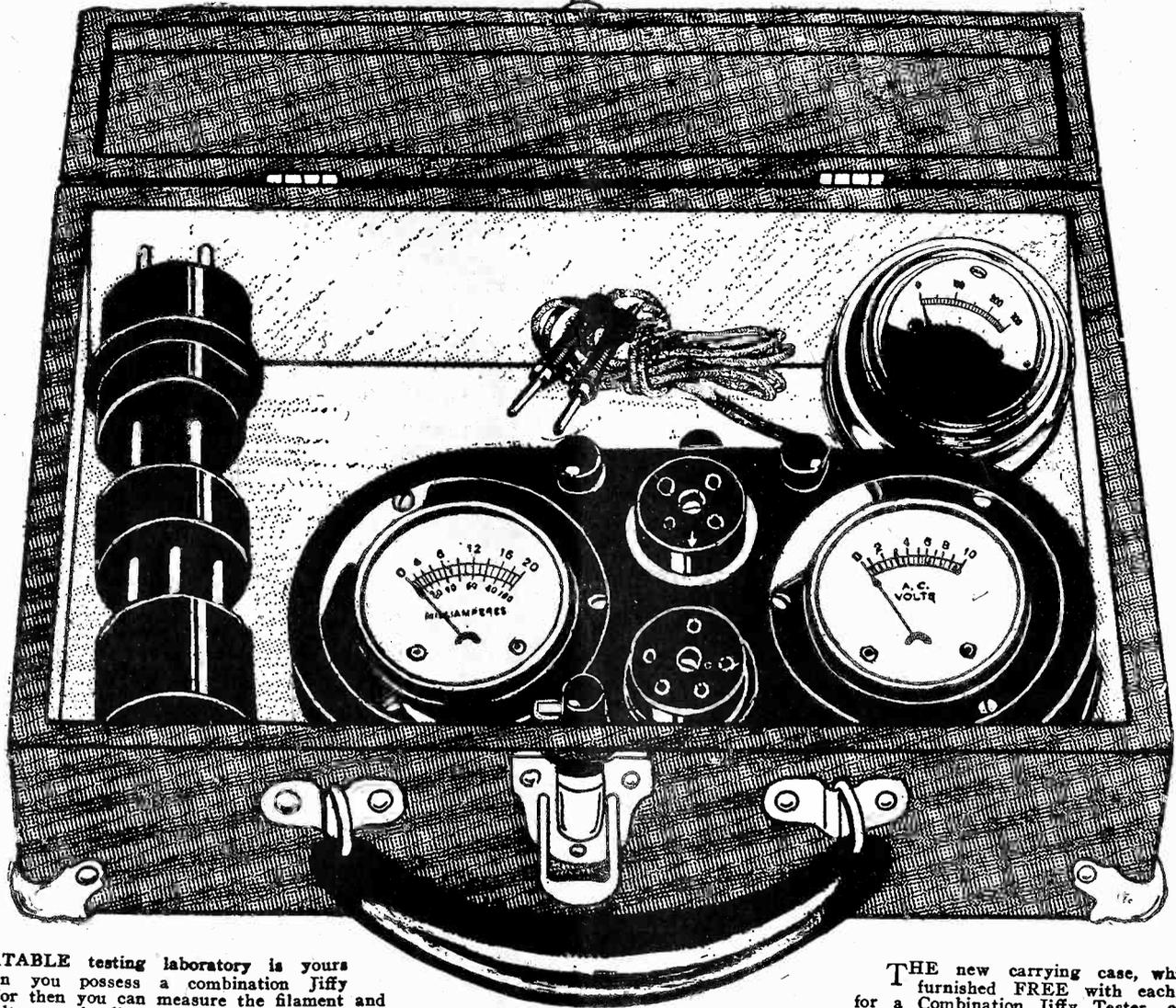
A PORTABLE testing laboratory is yours when you possess a combination Jiffy Tester, for then you can measure the filament and plate voltages of all standard tubes, including AC tubes, and all standard battery-operated or AC screen grid tubes; also plate voltages up to 500 volts on a high resistance meter that is 99% accurate; also plate current.
