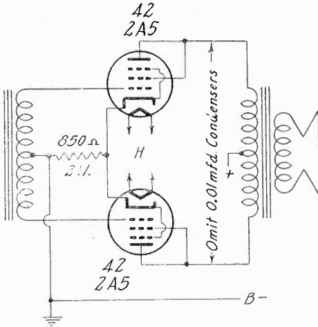
For triode connection screen and plate are tied together and the biasing resistor is raised to 850 ohms.
