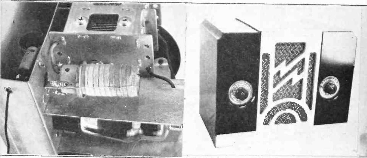
**I**N both the antenna and the interstage coil a high impedance primary is used in this five tube tuned radio frequency design. The results are excellent. In fact, the receiver works well enough to avoid trouble from WOR (now 50,000 watts) even in New York City, if a short antenna is used. Besides, the receiver does not oscillate even when a short antenna is used, which is an oddity, for it seems that most t.r.f sets suffer from this nuisance, which must be associated with poor design.
