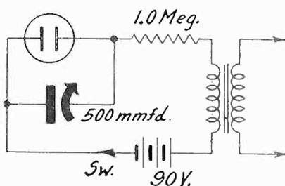
Intensity control is exercised at left by flipping the switch. The frequency remains practically unchanged. At right a variable condenser is used, for wide frequency change. The tubes must be of the type without limiting resistor built in.
