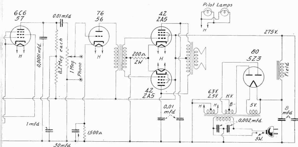
The detector, audio amplifier with pentode output, and rectifier, are shown above.
