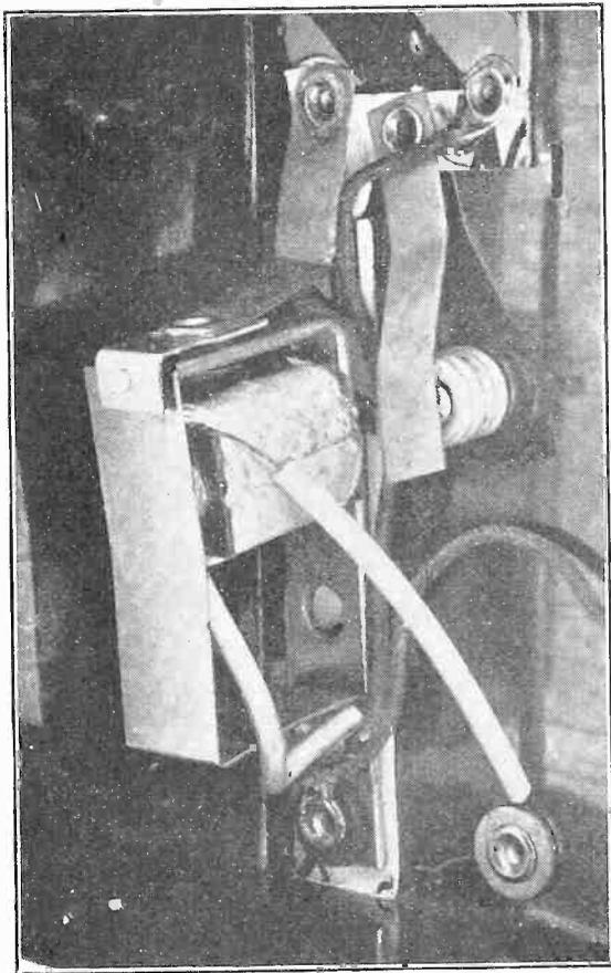
Close up of completed buzzer, showing make and break contacts on metal work at upper left.
