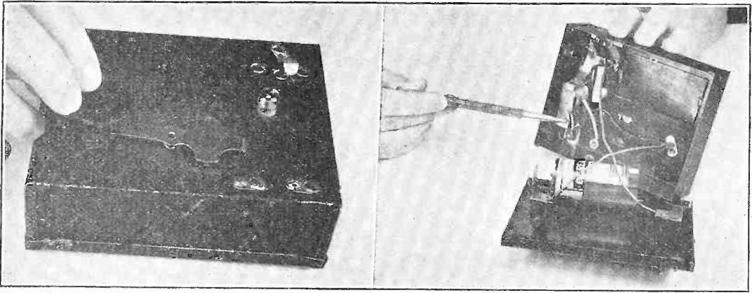
Upper left, completed apparatus in small metal box, with fingers properly placed on key knob for sending a practice signal. The little switch at rear of panel is used to change over circuit from buzzer to small flash lamp, thus giving visual signal, and no buzz. Pencil (right) points to "works" inside can and flashlight cells for supplying necessary electricity.
