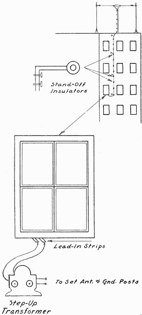
Typical doublet antenna installation for serving the occupant of an apartment.
