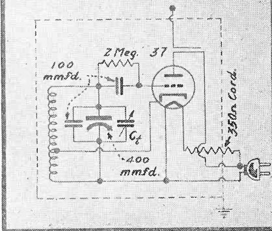
The box and the simple signal generator it contains. This generator works on a.c. or d.c. but has no modulation on d.c.
