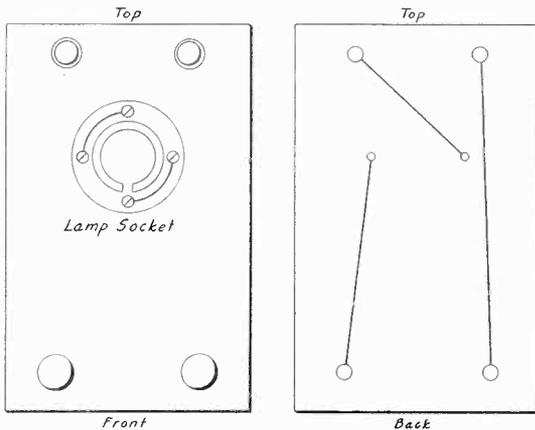
Diagram and top view. Condenser test post shorted, lamp is output meter.
