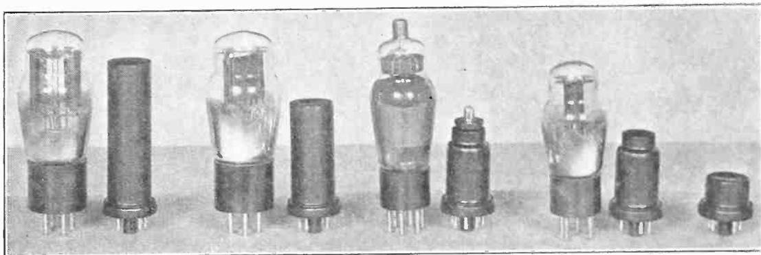
Contrast between the new metal radio tubes and glass-enclosed tubes of corresponding ratings. Left to right: rectifiers, power tubes, radio frequency tubes, small triodes, and, alone, the new duodiode, available only as a metal tube.
