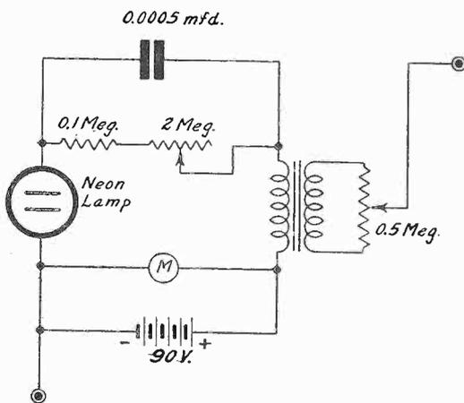
Variable frequency neon audio oscillators, with attenuation. The resistor is fixed, the condenser variable, at left, while at right the condenser is fixed and the resistor is variable. The meter should be left in circuit during operation of the oscillator, as any calibration would be upset by a small change in the applied voltage. One side of the output transformer may be grounded.
