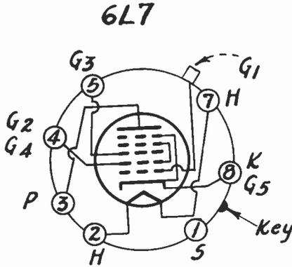
The internal arrangement of the elements of the 6L7 and the connections to the pins on the base.
