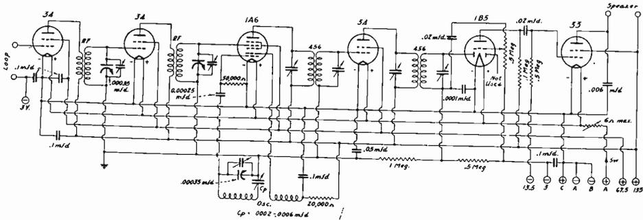
The circuit of the portable superheterodyne.
