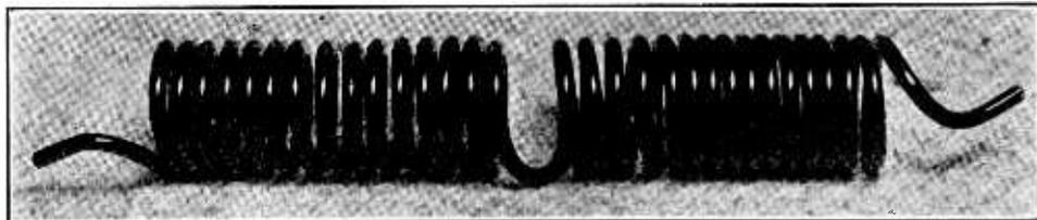
Coils for line filters may be wound in this elongated manner, using large diameter wire, No. 8 or No. 10. Another method is to wind on dowels.
