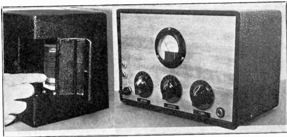
A small battery operated portable receiver for earphone use, wave bands changed by plugging in a single coil for each band. Note the hinged door permitting access to the coil socket for band shifting. The front panel controls may include a 35 mmfd. series antenna condenser, the one at extreme left on the panel.
