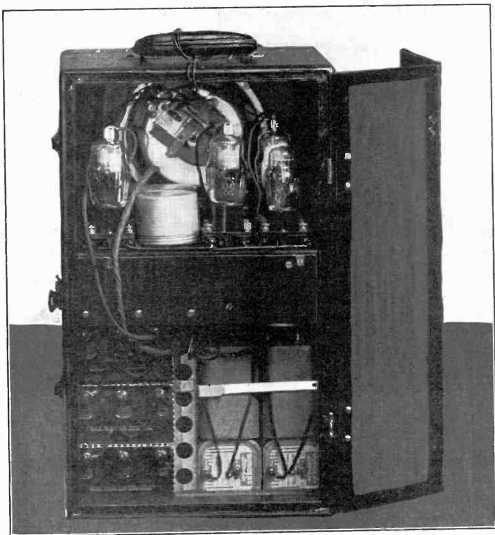
Rear view. The power supply is at the bottom, the chassis in the middle and the speaker at top.
