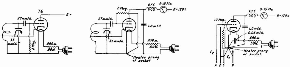
For operation on five meters the oscillator at left was used at one stage, but as a.c. was on the plate, oscillations ceased too soon, and little reduction of wavelength could be accomplished. Higher leak and inclusion of choke and by plate bypass condenser (center) improved matters. A nearly literal diagram is at right, AB, (C2), representing the grid condenser, and CD, (C1), the tuning condenser.
