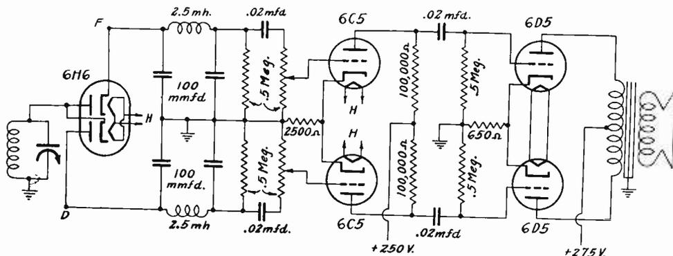
A complete diode detector and audio amplifier in which resistance-capacity coupling is used between the detector and the push-pull circuit. This is not strictly nonreactive, but can be made symmetrical.
