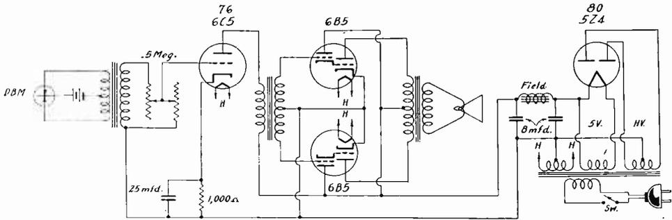
A small amplifier, using a 76 or 6C6 driver ahead of a push-pull 6B5 output, for double button microphone input.
