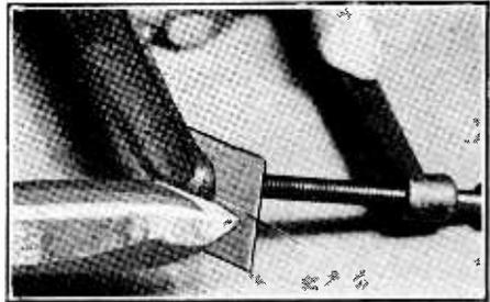
A needle may be used as pointer. The bracket is held in a C clamp and the needle is soldered to the bracket.
