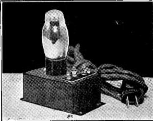
**Radio Design Field Supply Rectifier**
