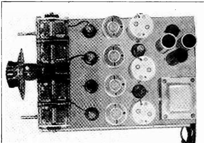
frequency have greater amplitude, posterior stages should have the shorter, more direct leads, and the chassis layout, though restricted in some respects, leaves open the choice of where particular stages are to go, so that the leads may be kept to minimum length for the stage hardest driven, and may be longer, if need be, for earlier stages.
