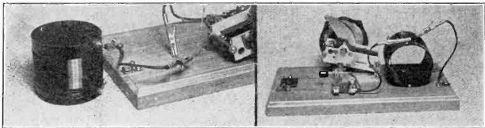
Only a crystal set, and nothing nifty about it, either. The simplest sort of receiver should be subjected to careful analysis for placement of parts, so that at least compactness and neatness will prevail, especially where the occupation of almost as much territory as an army would want in an enemy country doesn't help performance a bit.
