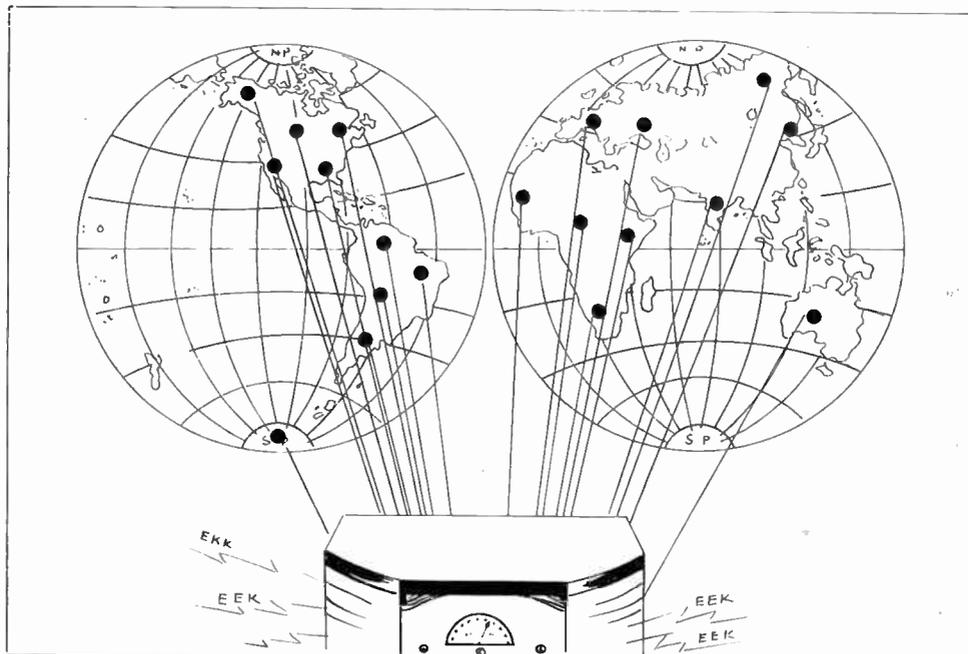
So many stations all over the world use short waves for long-distance broadcasting that it is inevitable on occasions that this multiplicity of radiation will produce interference in the receiver, such as squeals, or humming or singing tones. A tone control that reduces the high audio-frequency response may be adjusted to minimize this interference, but in general the nuisance has to be tolerated, or the set tuned to some other part of the dial.
