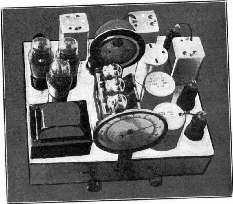
When the proper tracking is established, the dial readings are what they are and can not be changed, without going through the performance as recommended by Mr. Wheeler. This applies particularly to sets with frequency-calibrated dials. The standard broadcast band is considered. The short-wave and intermediate-short-wave bands needs not be given any thought, as the quantity of change of intermediate amplifier frequency is small compared to the station frequencies in those instances.
