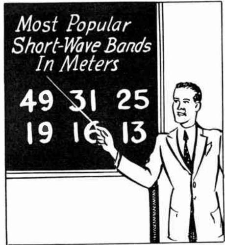
International entertainment programs are transmitted principally on wavelengths around 49, 31, 25, 19, 16 and 13 meters. Some dials do not carry wavelength designations, but frequencies instead. The approximate frequencies in megacycles would be, respectively, 6, 10, 13, 16 and 23. If the dial has only 0-100 designations, the dial positions for wavelengths or frequencies should be recorded on the basis of information announced from the stations.
