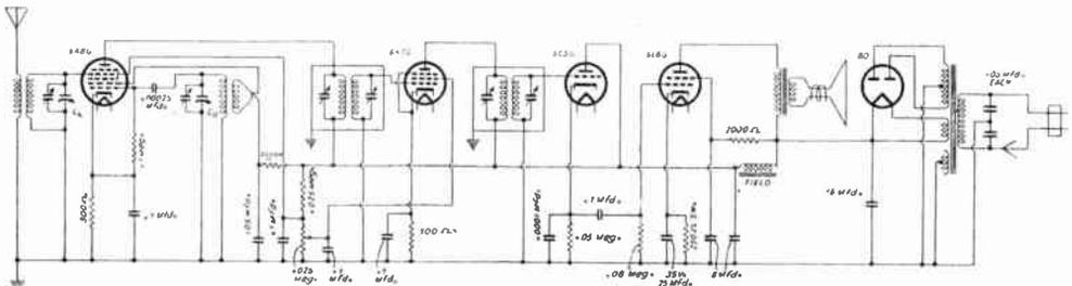
The alignment discussed applies particularly to padded oscillator circuit, and not to a set with tracking section (above).
