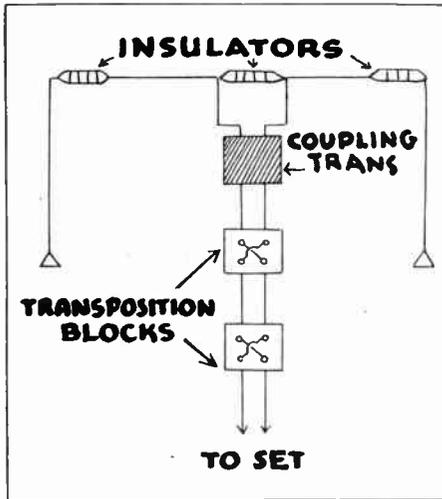
Special antennas of various types are on the market, to enable better reception of short waves. Not only may some stations thus be brought in with greater absolute volume, but also with less interference due to local noises. One system is to have a coupling transformer near the special antenna, with download consisting of two wires transposed every few feet, so no local noise is picked up by the lead-in. The download may be twisted pair instead.
