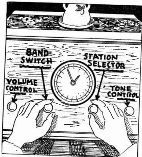
The four main controls on a receiver are the band switch, which determines the extremes of the frequencies or wavelengths that may be tuned in at a particular switch setting; the station selector, which makes the receiver responsive to some particular frequency within the band permitted by the switch setting; the volume control, for adjustment of the quantity of sound output; and the tone control, to enable alteration of the response characteristic to suit particular tastes of reproduction.
