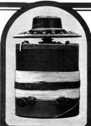
*Above is the wave trap as we made it with the Rathbun condenser and container. The photograph shows clearly how the forty-five turns of cotton-covered wire were wound on first and the six turns of the large stranded wire were wound over top of it.*
