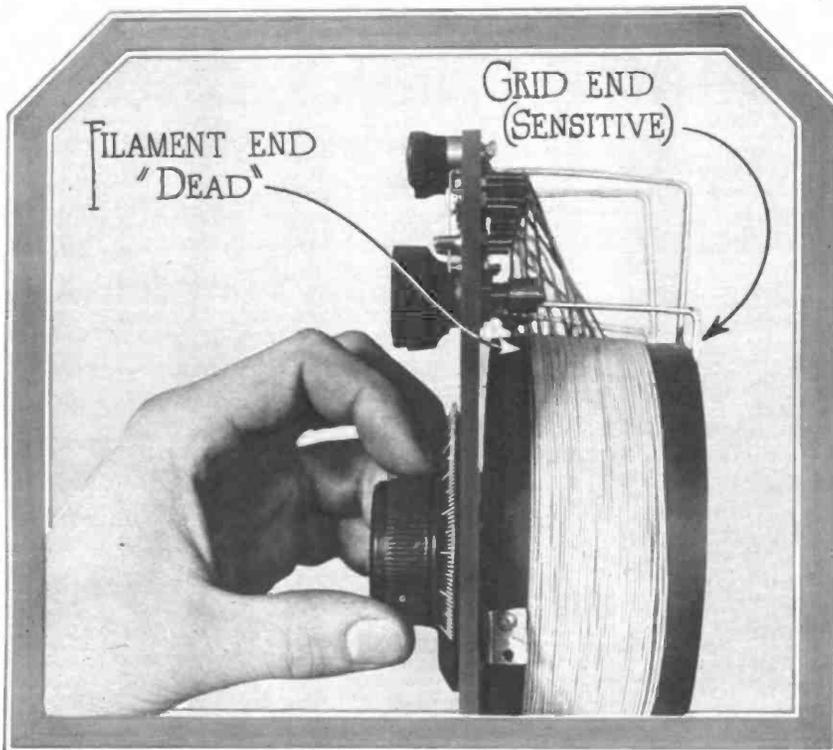
The coils are correctly mounted when the end which connects to the grid or grid condenser are farthest from the panel. The effect of the hand is not exerted on the front end of the winding since it is at ground potential.
