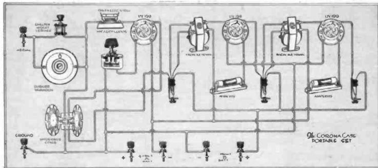
which is connected to the Variadon in what we call parallel—that is, one side of the midget is connected to one side of the Variadon and the other two sides are connected to each other.
