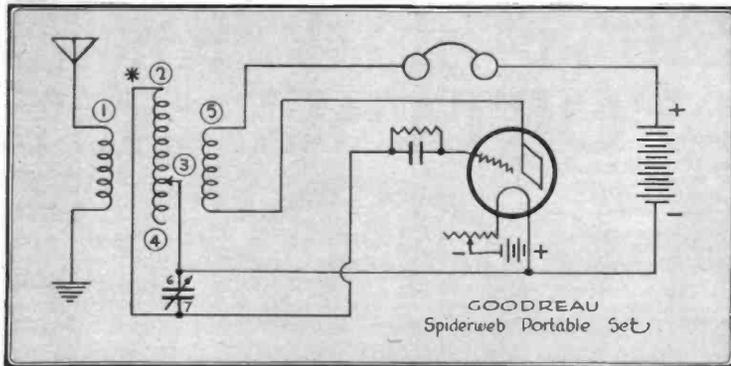
When using antenna or ground alone, connect at this point. When using both antenna and ground, connect as shown to primary coil
