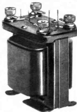
The wires extend through the Bakelite top, which affords perfect insulation, and are soldered to the terminals in plain sight, where they may be inspected. This also eliminates any possibility of breakage of transformer leads.
