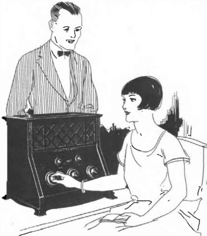
*WorkRite Radio-King*, a five tube (2 radio amplifier, 1 detector and 2 audio amplifier) super neutrodyne receiver. Beautiful mahogany cabinet, 22 in. x 20 in. x 14 in. This set operates with outdoor or indoor aerial and is highly selective. Long distance stations come in full and clear on the built-in loud speaker. Complete except tubes, batteries and aerial wire . . . \$220.
