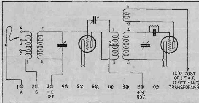
The wiring of the radio frequency and the detector circuits.
