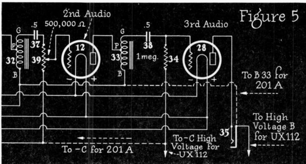
with impedance coupled audio amplification.
