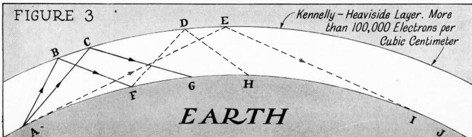
Based on the reflection theory the rays from the transmitter at point A are shown reflected downward by the radio roof and upward by the ground. The skipped distances are indicated.
