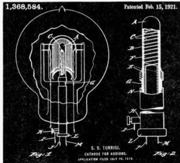
tungsten, the same as the filament and some difficulty was experienced in obtaining a copious supply of electrons because the construction did not permit the cathode to get as hot as the inside filament.
