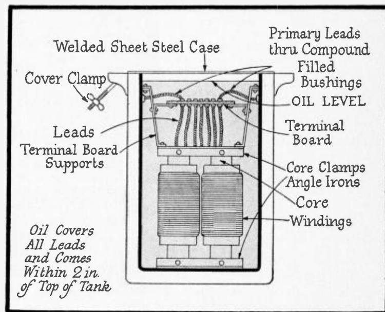
*Above is a sectional view of the kind of power-line transformers blamed by most radio fans for interference. Mr. Allen's article explains its construction and shows that most of such complaints are not justified.*
