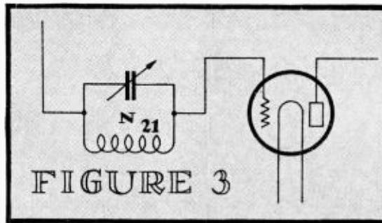
tem, such as a frame (loop aerial) and even allows the use of a special untuned aerial wire, without earth connection, as the sole stimulator. This diagram illustrates the 3-electrode tube 16 used without H. F. (radio frequency) oscillation. Its grid and filament are joined across the circuit 17, which corresponds with the "N" in Figure 1. One point of this oscillator is joined to a point in the stimulating circuit.
