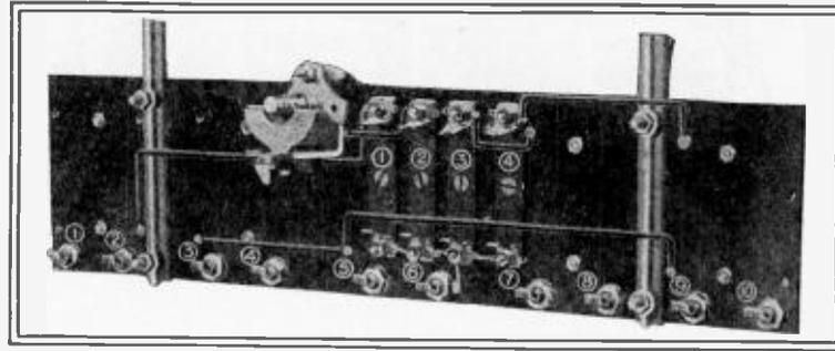
Bottom view of sub-panel illustrating correct wiring.
