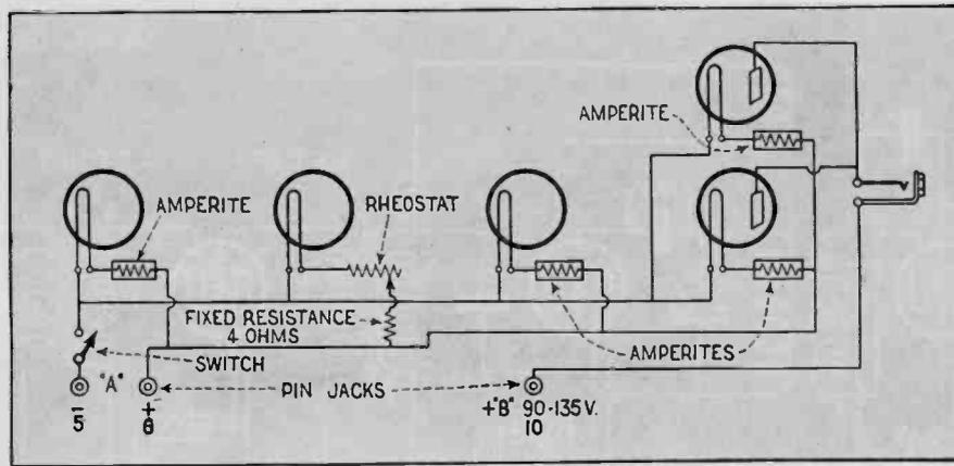
This diagram shows the complete wiring of the filament circuit.
