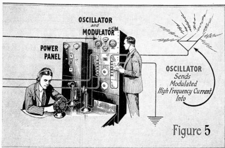
studio to the ether waves radiating from the broadcasting antenna.
