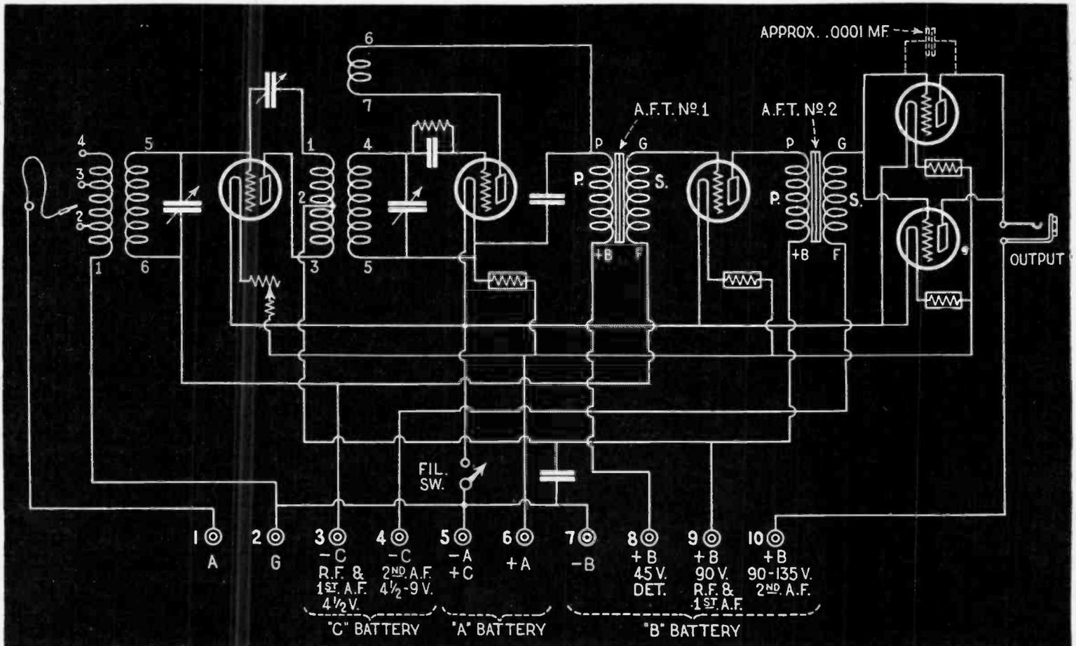
by tracing the path of the currents through the receiver. A stage of radio frequency amplification is used to increase the signal received in the antenna. This tube is neutralized to prevent radiation and annoying your neighbors.
