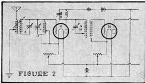
a means of separating or disassociating the receiving set proper—i.e., the tube amplifier—from the collecting system, or aerial; thus preventing the comparatively powerful currents flowing in the tube circuits from energizing the aerial and so forming a source of local reradiation or disturbance.
