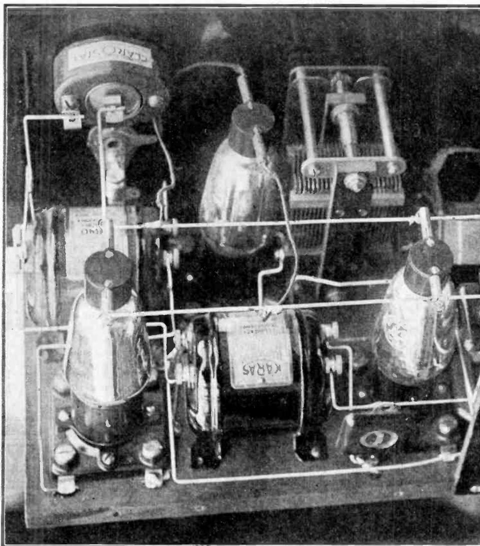
*The heater connections are made with clips soldered to little wire springs which are, in turn, soldered to long pieces of bus wire. Note that the heater element connections come out at the top of the tubes.*
