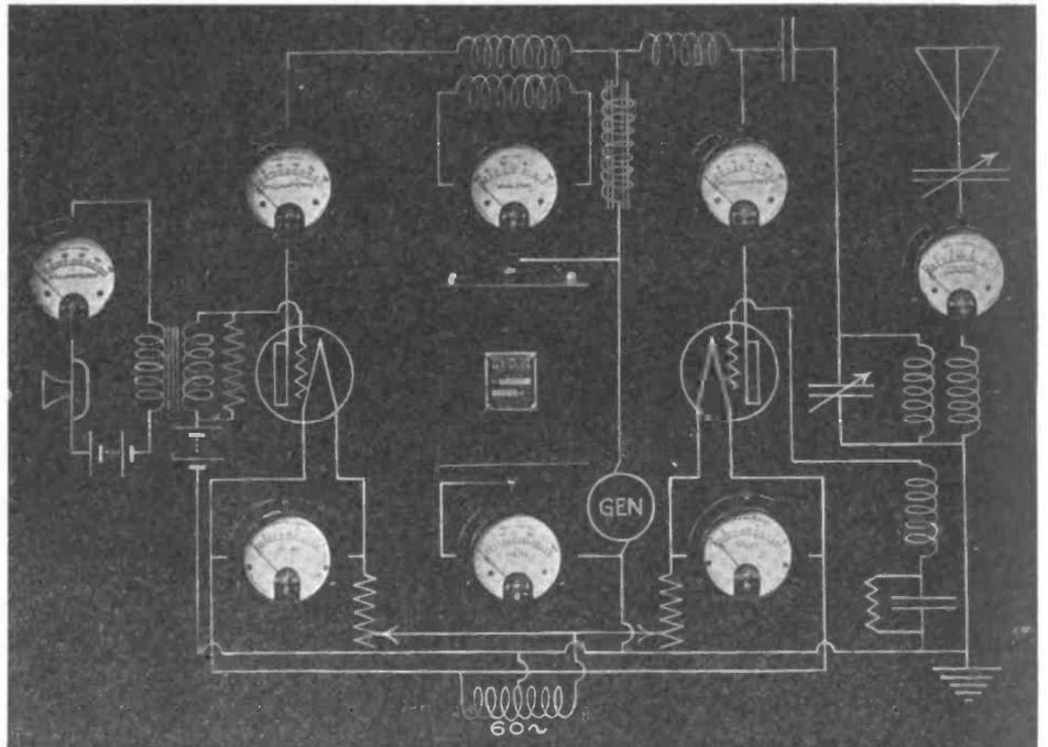
Graphic Placing of Jewell Instruments on Radiophone Hook-up
