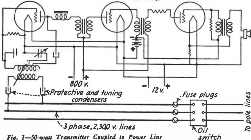
Fig. 1—50-watt Transmitter Coupled to Power Line
