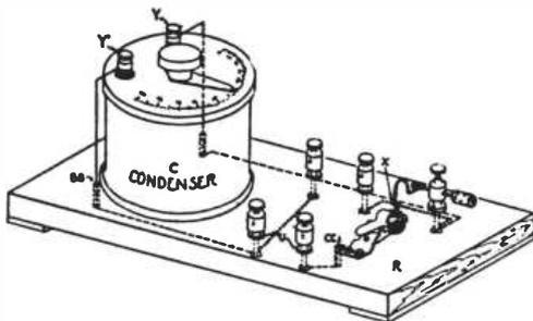
Fig. 6—Two-Circuit Tuner Connections
