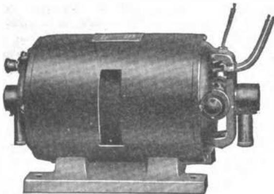
Fig. 70. Two Bearing Single Unit Motor Generator
