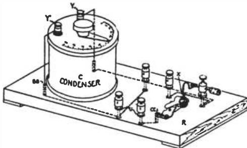
Fig. 6—Two-Circuit Tuner Connections
