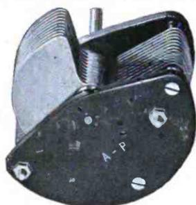
A quality product. Panel type. Plates of No. 20 heavy gauge aluminum. Plate separators gauged to 1/2 of 1-1000 of an inch, machine turned and nickel plated shaft. Top and base of 1/4-inch sheet Bakelite Di-electro. Projecting shafts supplied on request.
