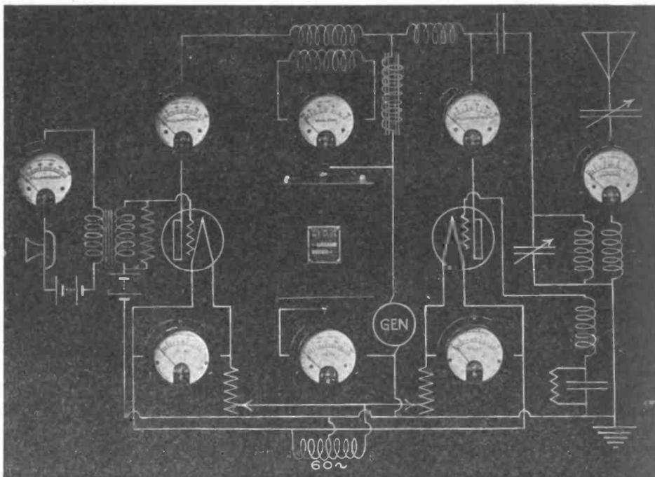
Graphic Placing of Jewell Instruments on Radiophone Hook-up
