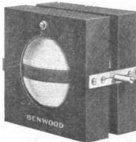
These variometers cover a wave length range of 150 to 650 meters when used in conjunction with the average variocoupler. The features are, minimum distributed capacity, minimum distance between stator and rotor, large size wire on both coils, positive contact bearings and properly designed mechanically as well as electrically.
