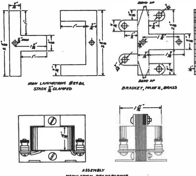
Fig. 26. Assembly of Modulation Transformer
