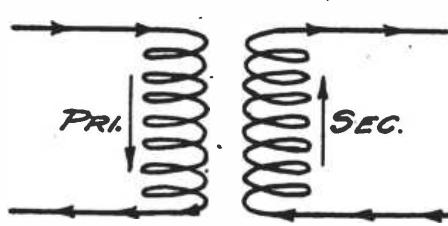
Fig. 8. How Downward Current in Primary Induces Upward Current in Secondary
