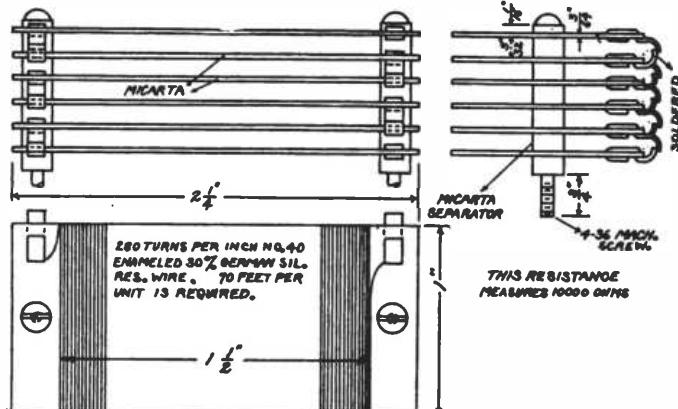
Fig. 27. Details of 10,000 Ohm Grid Leak
