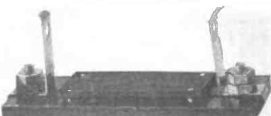
Mica Grid Condenser and Grid Leak Mountings
