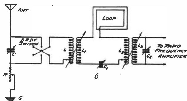
Fig. 4. Loop with Winding at Right Angles to Direction of Line with Direction of Wave Travel. No Signal.
