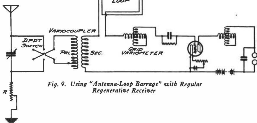
Fig. 9. Using "Antenna-Loop Barrage" with Regular Regenerative Receiver
