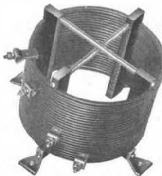
Standard size as shown consists of 25 turns of edgewise wound soft drawn copper ribbon  $\frac{3}{8}$  inch in width,  $\frac{1}{16}$  inch in thickness and the turns are SEVEN INCHES in diameter.
