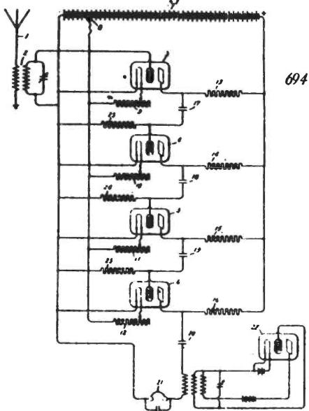
22 and 23. A contact 20 is also arranged on the sending key 17 so that when energy is radiated, the e.m.f. supplied to motor 9 is increased so as to prevent a sudden drop in speed due to sudden increase of load.
