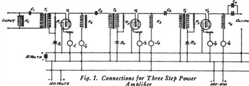
Fig. 1. Connections for Three Step Power Amplifier
