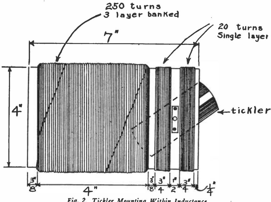
Fig. 2. Tickler Mounting Within Inductance
