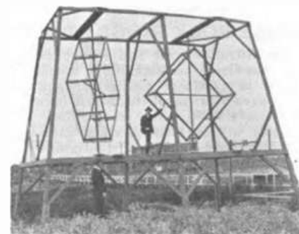
A 5,000 mile aerial! These loops are used for receiving. By means of gears and shafting the loops can be rotated by the operator at his desk (Kolster loop circuit).
