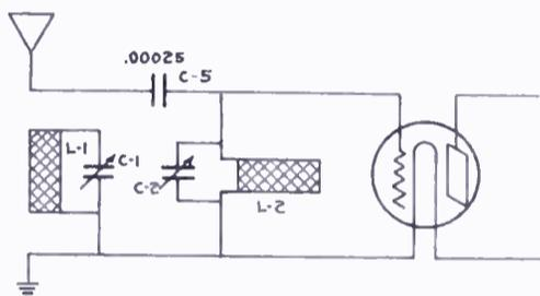
Fig. 1. Selector for Single-Circuit Set
