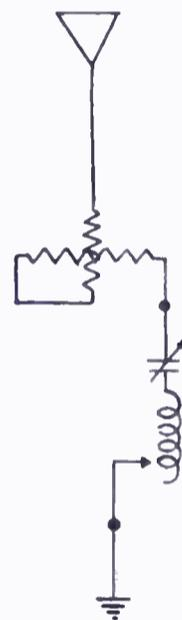
Fig. 4. Circuit with Variometer
