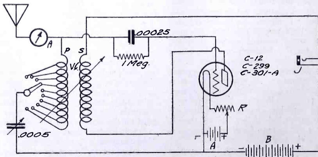
Fig. 1. Hook-up for Groundless Receiver
