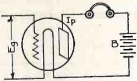
Fig. 1. Elements of Detector Tube
