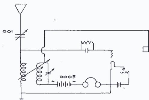
Fig. 1. Hook-up for One-Tube Receiver
