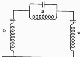
Fig. 4. High and Low-Pass Filter
