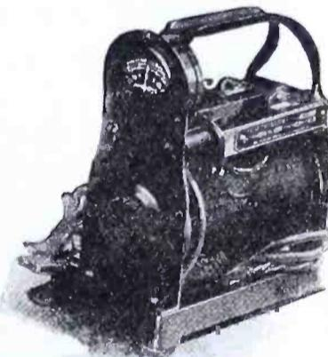
Recent developments in the radio field instigated new improvements in the design of the Sterling Rectifier. The 5 ampere maximum charging rate has been adopted and with it the number of contacts has been reduced to one, offering more simplicity and ease of adjustment. Special wear-resisting carbons of large cross section area prevent freezing and sticking. Quiet in operation. No consideration of polarity necessary in connecting to battery. Cannot overcharge battery because of tapering charge.
