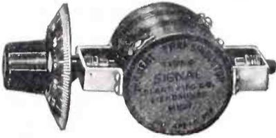
The "Transinductor" is a new type of variable transformer which gives selective tuning and high amplification by means of a one-dial control of the magnetic inductance, capacity and iron flux. It is equally well adapted for either radio or audio-frequency amplification with any make of tube.
