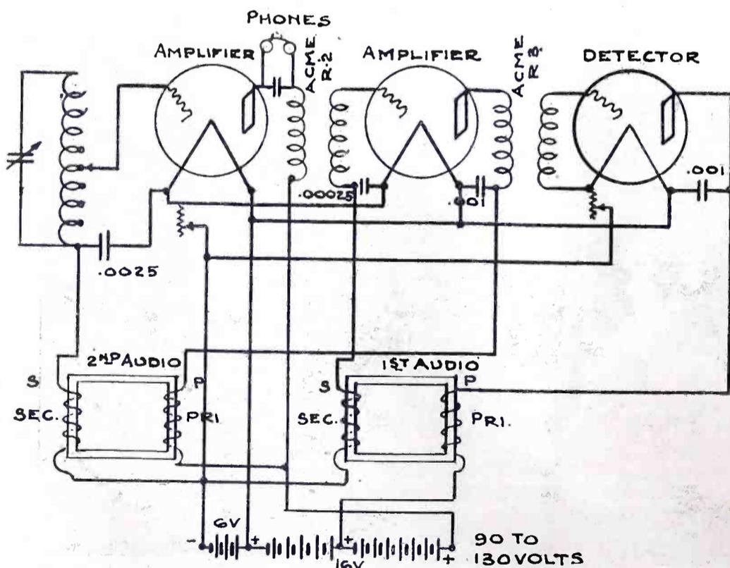
Fig. 3. Wiring Diagram for Grimes Inverse Duplex
