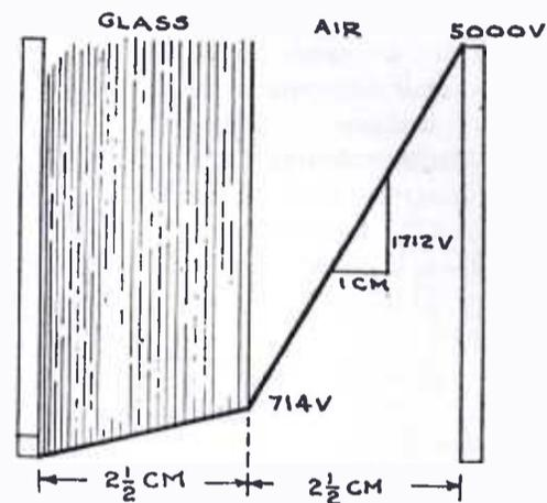
Fig. 2. Voltage Distribution Through Non-Homogeneous Insulation
