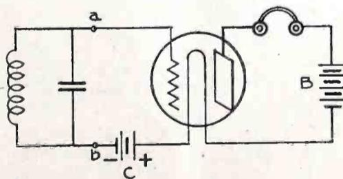
Fig. 4. Wiring Diagram of V. T. Detector Circuit With Grid Biasing Battery
