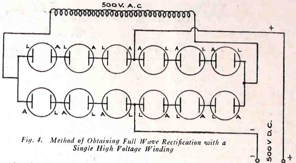
Fig. 4. Method of Obtaining Full Wave Rectification with a Single High Voltage Winding
