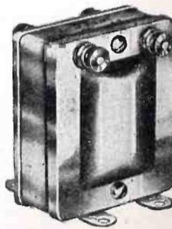
The National audio-frequency transformer is claimed to give great volume and fine tone quality, especially for low notes; shell type laminated silicon steel core assures minimum core loss and accurately wound coils give low distributed capacity; completely inclosed in metal case to eliminate stray fields; extra long binding posts plainly marked; made in  $3\frac{1}{2}$  to 1 and 6 to 1 ratios.
