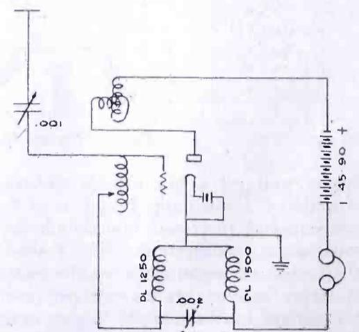
Fig. 5. Adaptation to Single-Tube "Super"
