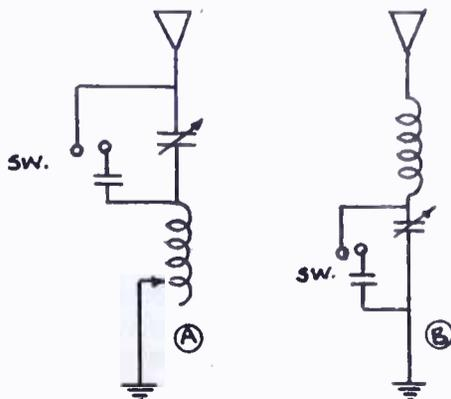
Fig. 3. Use of Shunt Condenser
