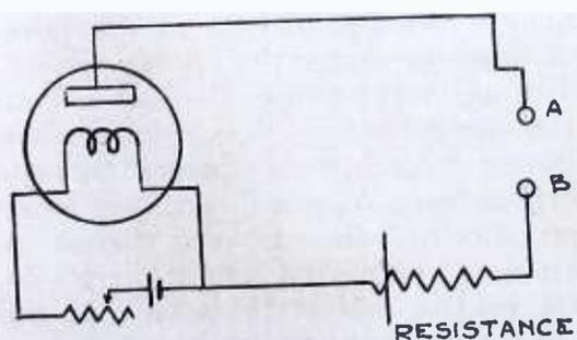
Fig. 2. Gas Filled Tube Rectifier
