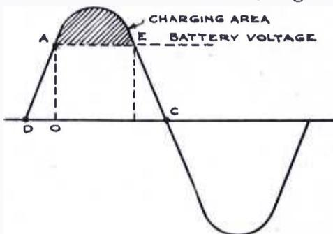
Fig. 10. Diagram of Charging Cycle
