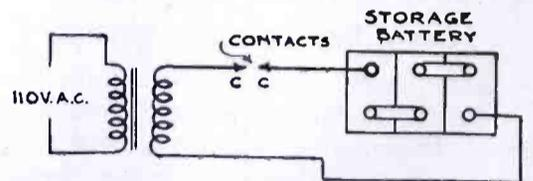
Fig. 9. Elementary Circuit for Vibrating Contact Charger
