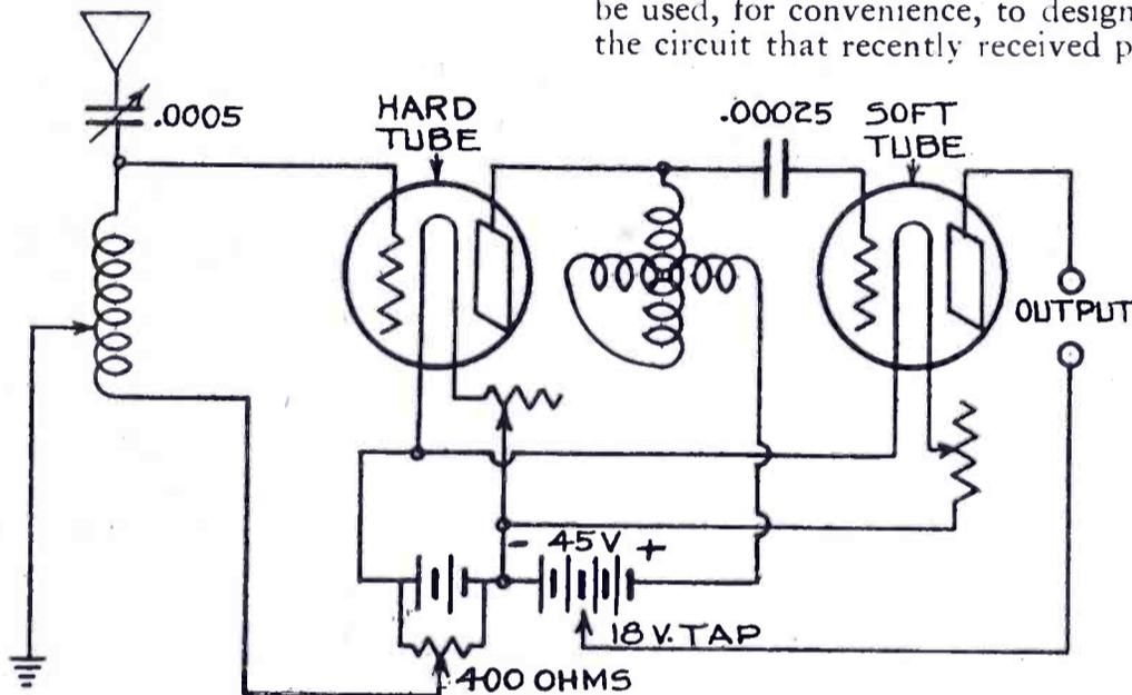
Fig. 1. Connection for a One-Step R. F. Amplifier
