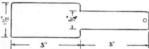
Fig. 2. Dimensions of Plates for Chemical Rectifier
