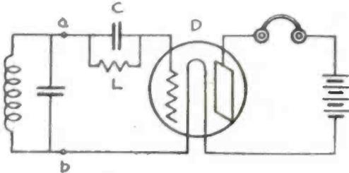
Fig. 6. Detector Circuit With Grid Condenser
