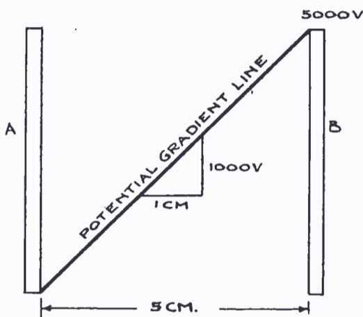
Fig. 1. Voltage Distribution Through Homogeneous Insulation
