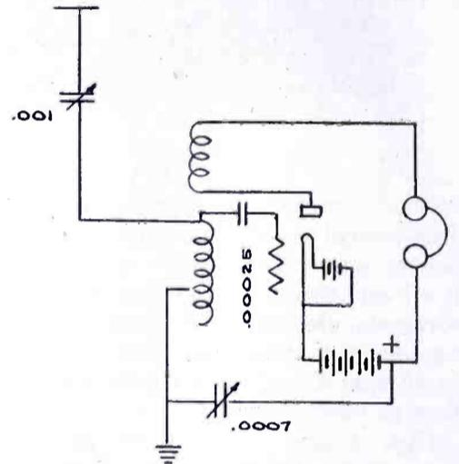
Fig. 4. Adaptation to Tickler Feed Back Circuit
