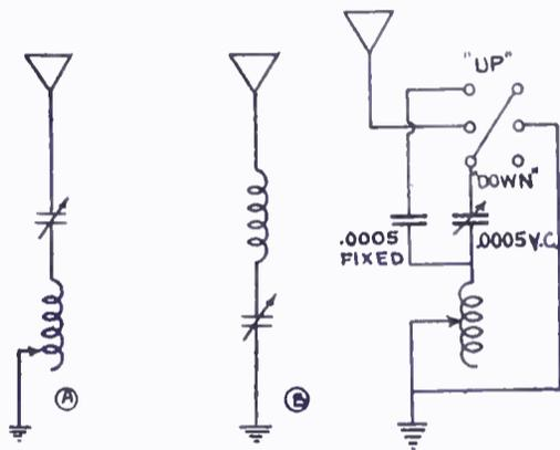
Fig. 1. Condenser Position in Primary Circuit
