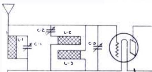
Fig. 2. Selector for Double-Circuit Set
