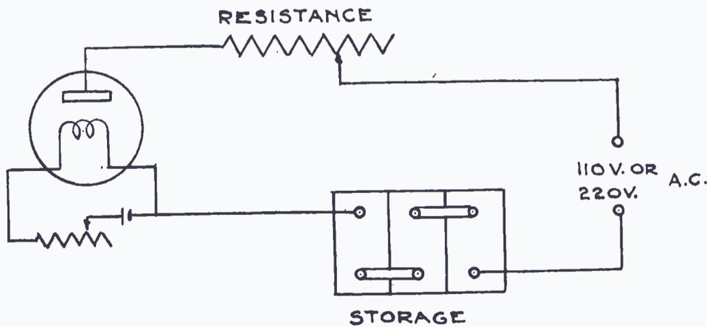
Fig. 5. Connection of Battery to Rectifier
