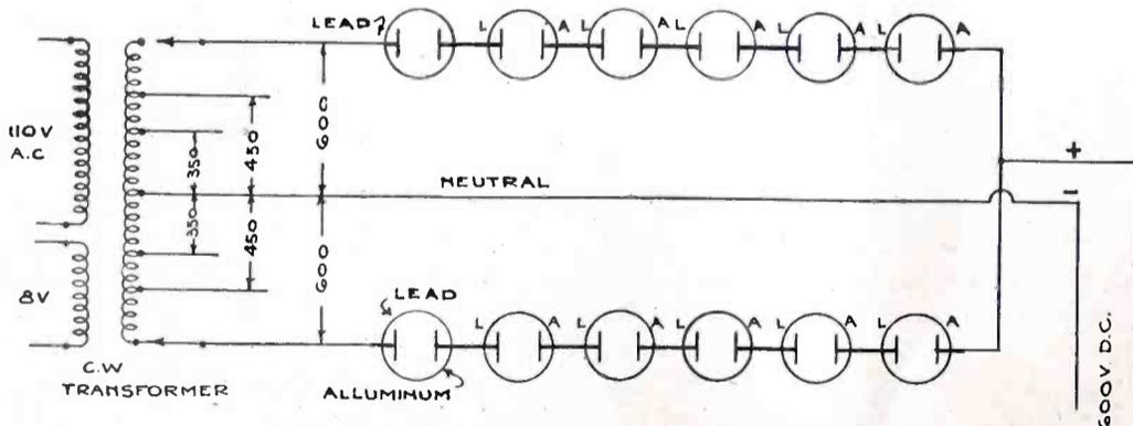
Fig. 3. Connections for Electrolytic Rectifier
