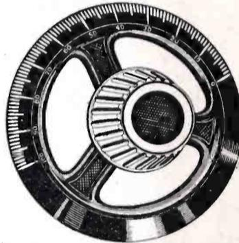
The Frost bakelite spider dial is designed to permit close tuning without vernier attachment; the beveled edge is of the conventional type, but the spider or yoke center and the fluted knob make it easy to grip; numbers and divisions are filled with white enamel, fitted with  $\frac{3}{16}$  or  $\frac{1}{4}$  in. brass bushing with set screw; made with  $2\frac{1}{2}$  or 3-in. dial.
