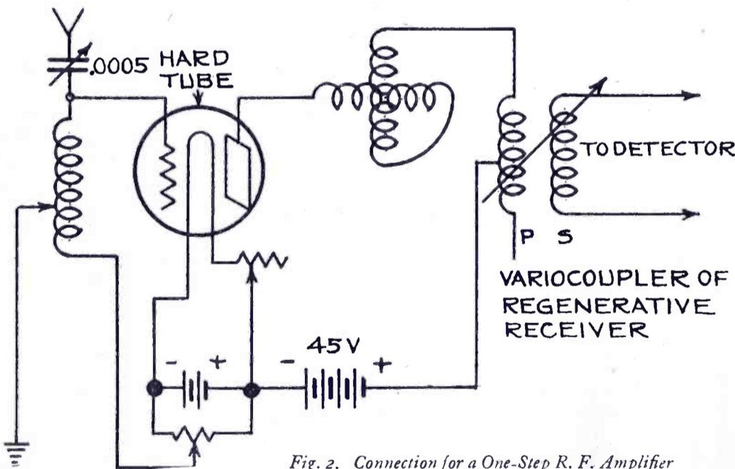
Fig. 2. Connection for a One-Step R. F. Amplifier
