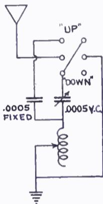
Fig. 2. Connection Diagram for D.P. D.T. Switch
