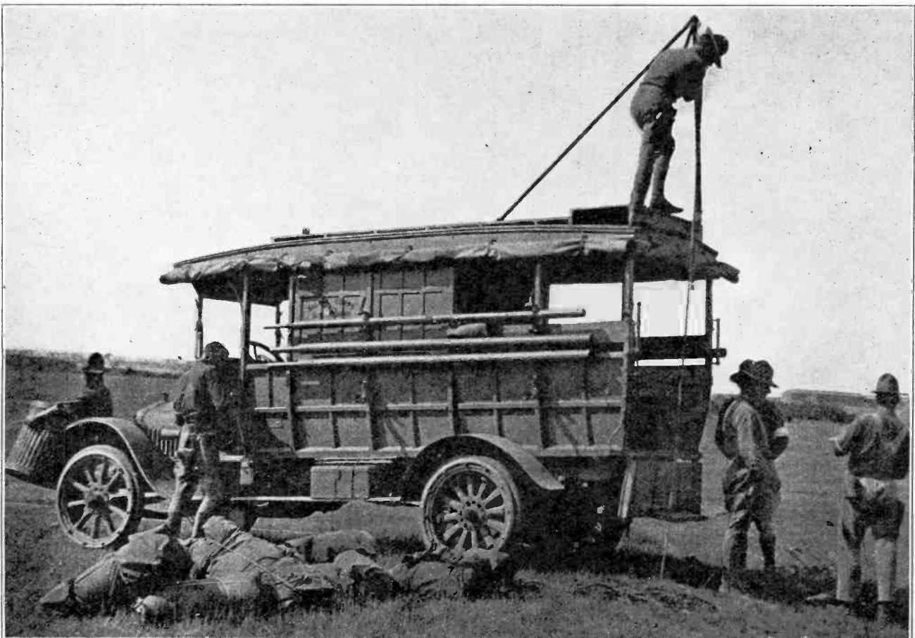
Radio Tractor Used to Communicate With Flying Airplanes During Army Tests at Panama
