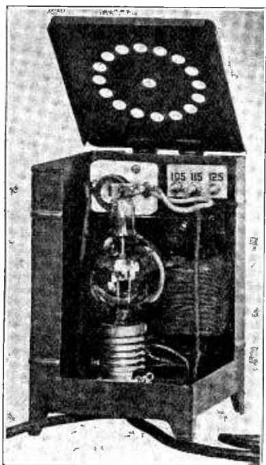
Fig. 7. Tungar Battery Charger
