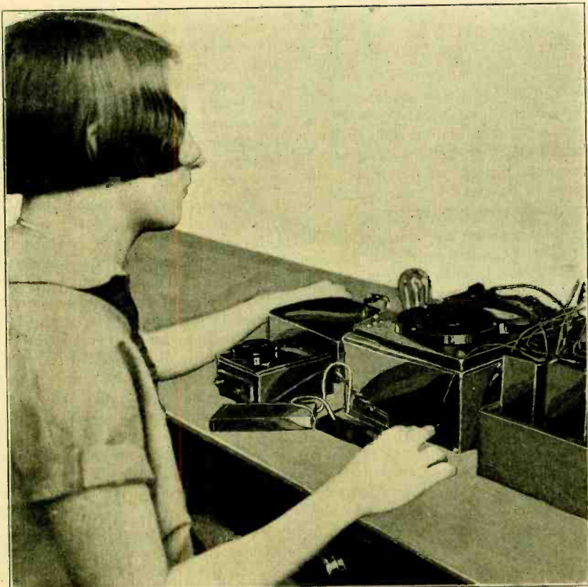
Testing a Condenser for Voltage Flash, Capacity and Leakage Resistance.
