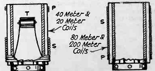
Fig. 2. Coil Winding Details.
