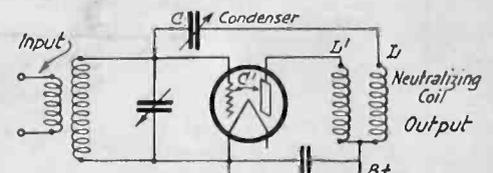
Fig. 3a. Hazeltine Method of Control.
