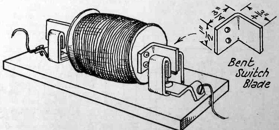
Fig. 2. Method of Mounting R.F. Choke.
