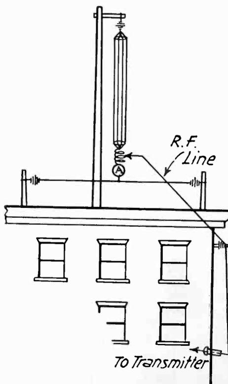
Fig. 2. Position of Antenna Receiver to Radio Frequency Feeder.
