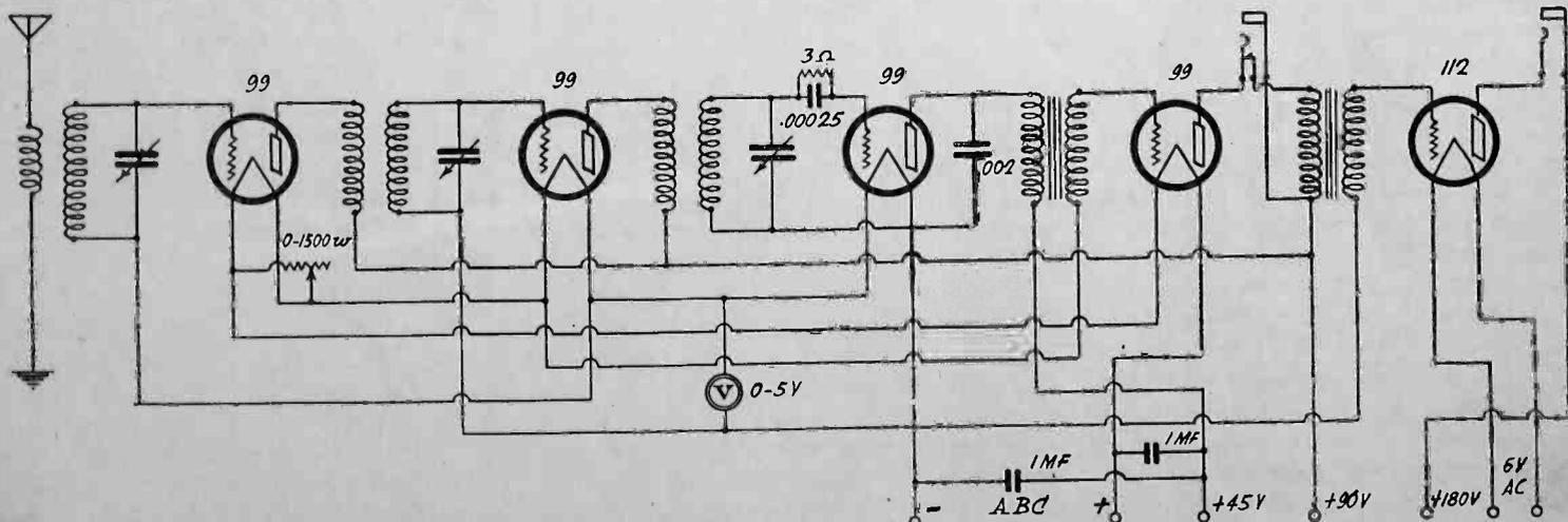
Fig. 2. Five Tube Receiver of Fig. 1 Rewired for Series Filament Connection.
