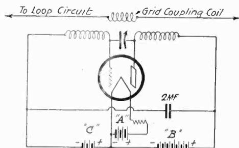
Fig. 3. Oscillator Used in Best Superheterodyne, with Series Condenser.
