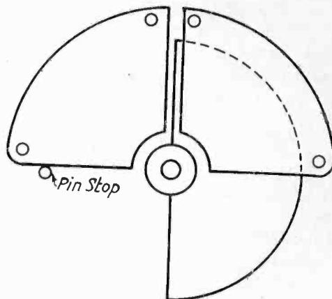
Fig. 2. Sectionalized Stator Plate of Directional Balance Condenser.
