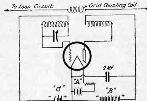
Fig. 2. Tuned Grid Oscillator, With Fixed Plate Coil.
