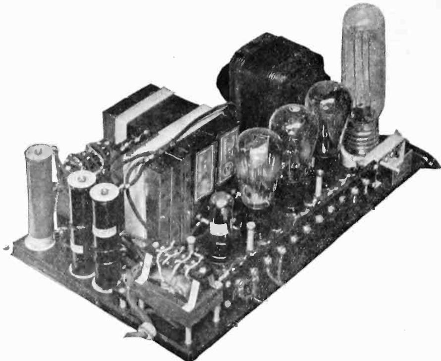
Fig. 2. Rectifier-Amplifier Assembly, Showing Constructional Details.
