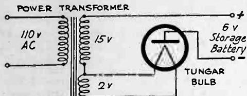
Fig. 1. Wiring Diagram for Two-Ampere Battery Charger.
