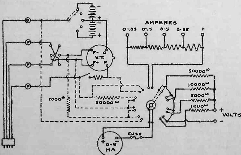
Fig. 2. Circuit Diagram of Testing Instrument.
