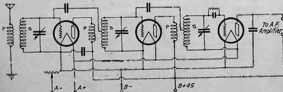
Fig. 2. Conventional Neutrodyne Circuit.
