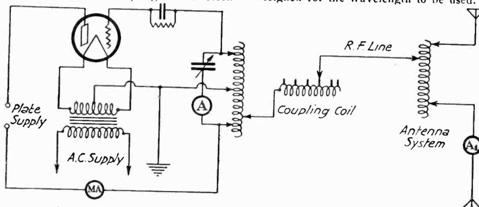
Fig. 1. Method of Connecting Transmitter for Reactance Coupling.
