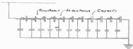
*Multi-Gap Lightning Arrester and Equivalent Electrical Circuit.*
