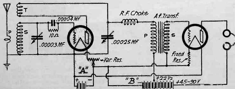
Fig. 1. Circuit for Short-Wave Receiver.
