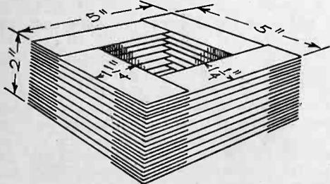
Fig. 2. Dimensions of Core for Battery Charger Transformer.
