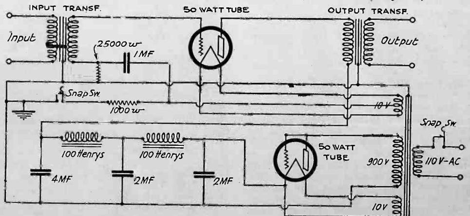
Fig. 4. Circuit for 50 Watt Power Amplifier.
