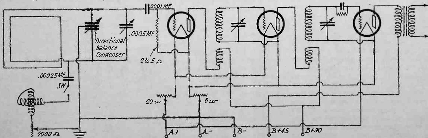
*Fig. 1. Circuit Arrangement for Directional and Uni-Directional Receiver.*
