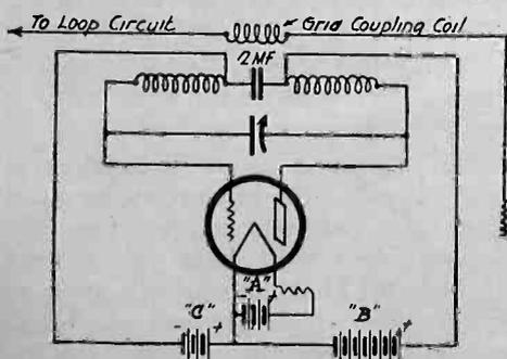
Fig. 1. Oscillator Circuit Most Frequently Used.
