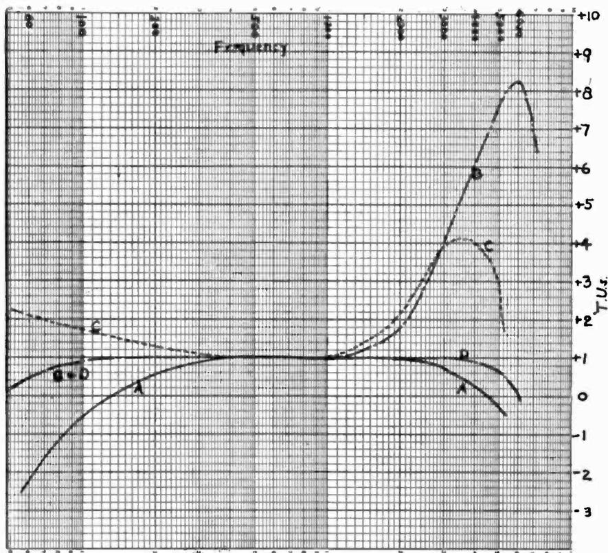
Fig. 3. Effect of Different Impedances on Audio Frequencies
