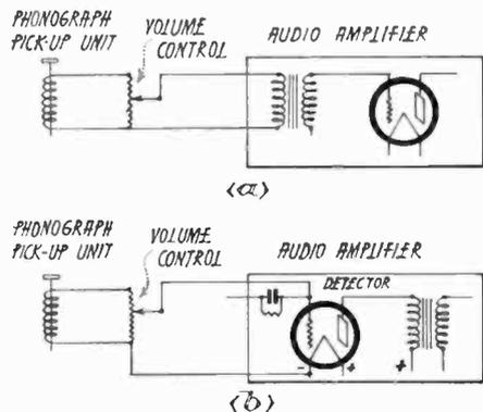
Fig. 1. Usual Methods of Connecting Pick-up Unit
