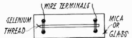
Fig. 1. Construction of Selenium Cell
