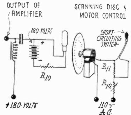
Fig. 1. Circuit Diagram of Television Receiving Equipment
