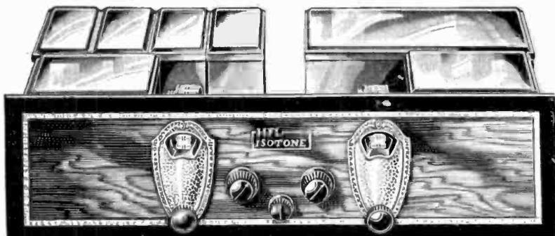
**Unlimited Range.** This excellent instrument employs practically every new engineering feature known to radio science. The range of the Isotone is almost unlimited. The three-stage screened grid amplifier having the unusually high gain of sixty-five per stage can be hand tuned by the operator which results in a perfectly balanced instrument. The 450 kilocycle amplifier allows absolute one spot tuning.
