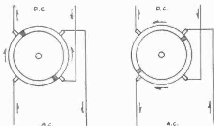
Fig. 1. Commutator Positions
