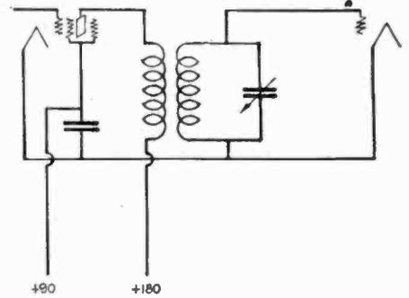
Fig. 3. a. R. F. Circuit Connections for Screen-Grid Tube with Conventional Transformers
