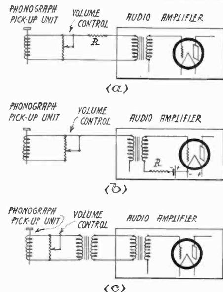
Fig. 4. Suggested Connections for Pick-up Unit. (In 4b the volume control resistance should be connected to ground.)
