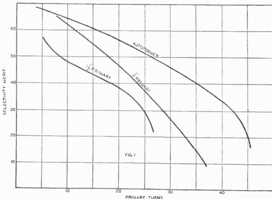
Fig. 4. Selectivity Curves for Three Types of Transformers
