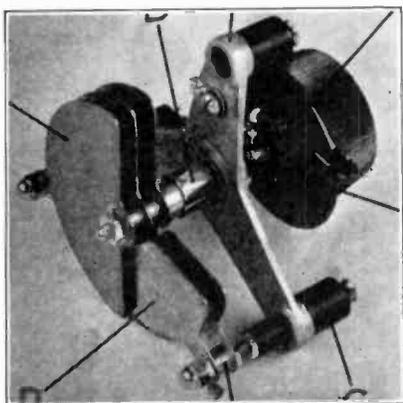
model illustrated has a maximum capacity of 54 mmfd. The capacity of the two-plate model may be regulated by moving the stator plate, thus giving a widespread tuning range.
