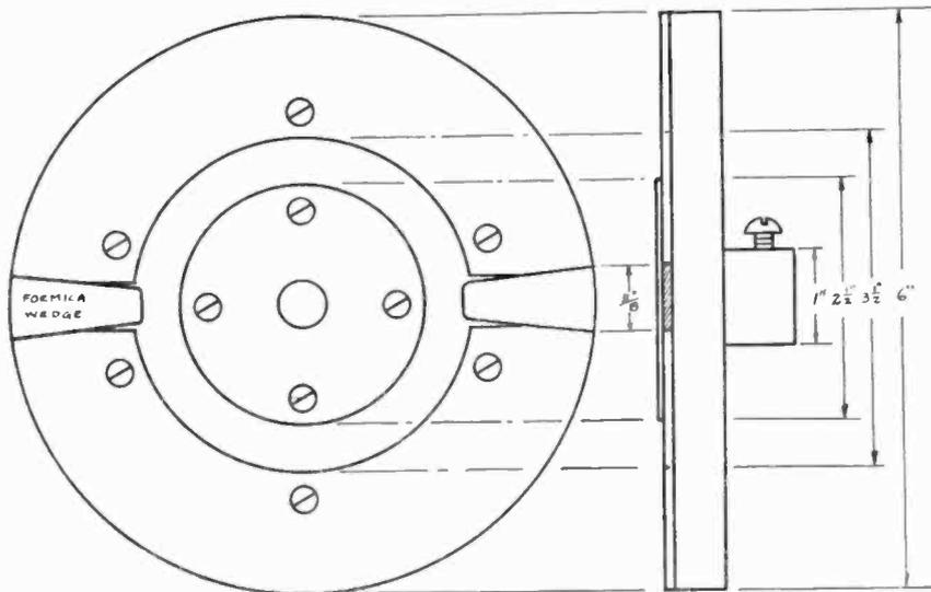
Fig. 3. Commutator Disc
