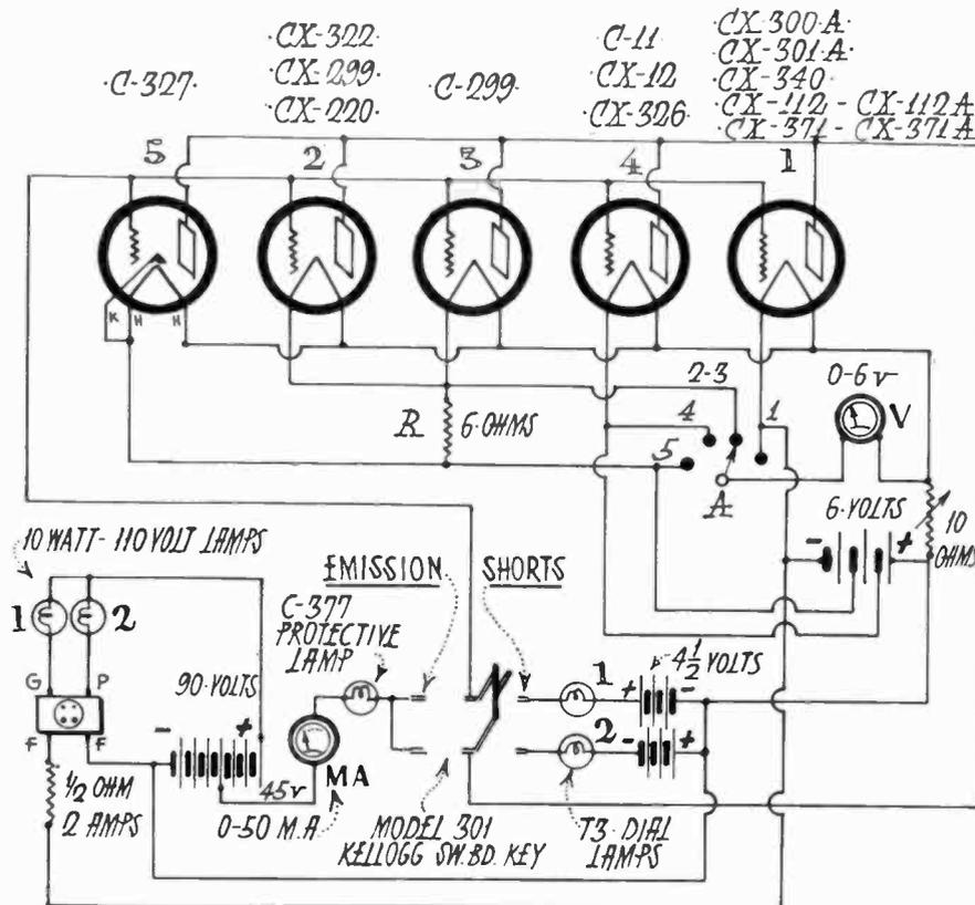
Fig. 1. Circuit Diagram of Complete Tube Tester
