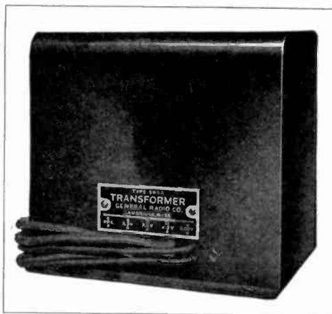
The General Radio Type 565 Power Transformers consist of two models for both half and full-wave rectification utilizing the 281 type of rectifier tube. The Type 565-A Half-Wave Transformer illustrated consists of one 600-volt secondary, two secondaries of 7.5 volts and one of 2.5 volts. It is designed for 105 to 125-volt, 50 to 60-cycle lines.
