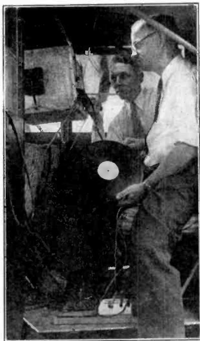
Picture Transmitting Equipment in Plane
