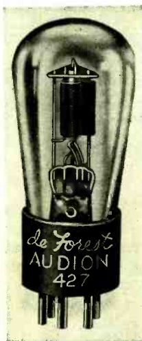
A humless Heater Tube De Forest Audion 427
