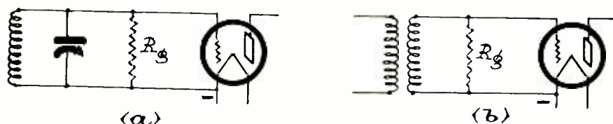
Fig. 2. Effective Shunted Resistance Caused by Grid Current in R.F. and A.F. Amplification Circuits
