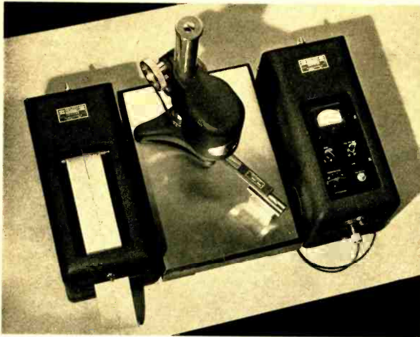
Fig. 1. A complete Surface Analyzer for measuring surface roughness. From L to R, direct-inking oscillograph, drive head with pickup arm resting on specimen, surface plate and calibrating amplifier.
