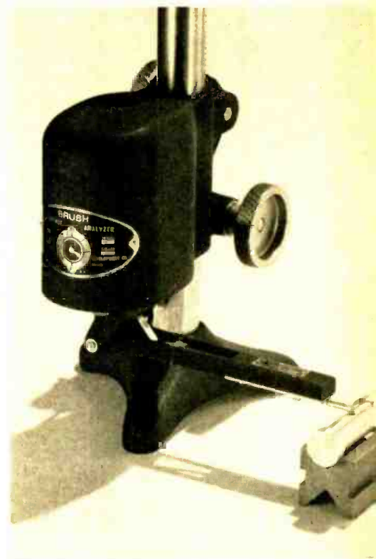
Fig. 3. Pickup arm rotated 90° to facilitate the measuring of intricately shaped surfaces.
