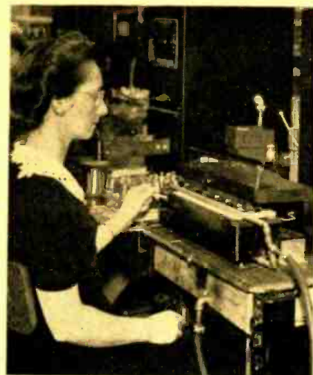
An electronic-type power oscillator, with fixture for soldering crystal units used for radio equipment.
