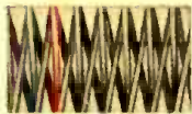
KOOLOHM interleaved winding—the perfect Ayrton-Perry type. Resistors are available having negligible inductance, even at 50 to 100 Mc.!
