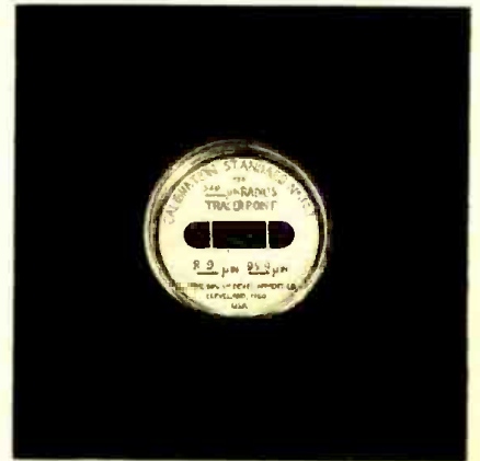
Fig. 4. Glass calibration standard for calibrating Surface Analyzer. Scratches appear above white parallel lines.
