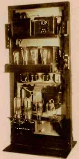
The new 50 watt Powerizer amplifier incorporates two UV-845 power tubes and two UX-866 mercury vapor rectifier tubes. Full wave rectification is used. This new Radio Receptor Company's product is of the new three unit panel construction. The amplifier may be used in various combinations with microphone pre-amplifier and radio or phonograph input.
