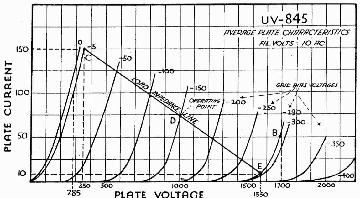
Fig. F. Modulator Load Impedance Line Drawn on the Plate Characteristic Curves of a Type UV-849 Tube.
