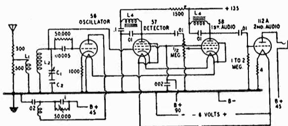
Fig. 1. The Special Heterodyne Circuit. L<sub>1</sub>, L<sub>2</sub>, L<sub>3</sub>—Windings of plug-in coil, see Fig. 3. L<sub>4</sub>—Iron core coil tuned to 800 cycles. C<sub>1</sub>—50 ufd. band-spreading condenser. C<sub>2</sub>—100 ufd. tuning condenser. (The band-spreading feature may be omitted or obtained in any of the usual ways.)
