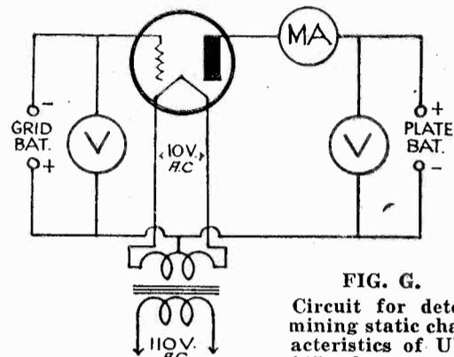
FIG. G. Circuit for determining static characteristics of UV-845 tube.
