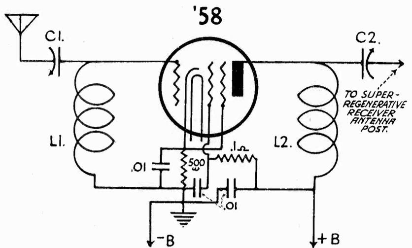
C1 & C2—Semi-variable 25 mmfd. max. (trimmer type condensers)
