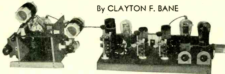
A complete medium-power transmitter with 47 oscillator, 865 doubler-buffer, 210 buffer and 800 amplifier. The 800 stage can drive an HK-354 Gammatron with ease.
