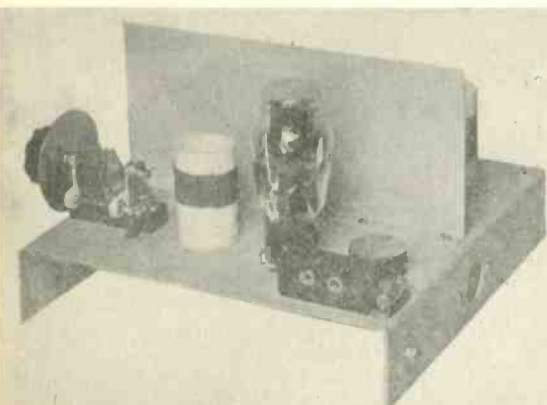
A One-Tube Xtal Transmitter to which an amplifier stage can be added at any future time.
