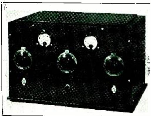
Not a receiver, but the r.f. end of a 40 watt, 160 meter phone transmitter.
