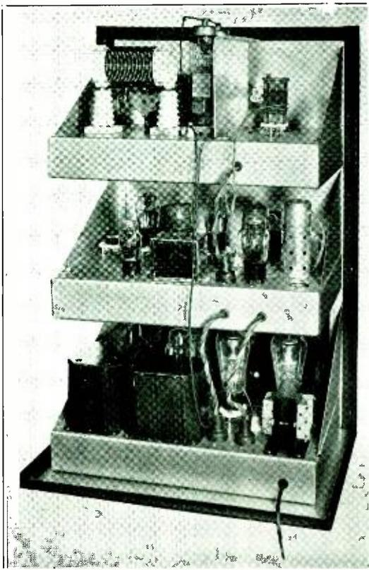
Showing interior construction of the transmitter. It is entirely self-contained.
