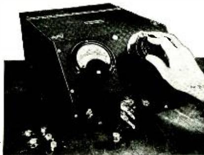
The QX-Checker is a companion instrument of the Q-meter in general use in well-equipped laboratories and engineering departments. This new instrument is intended for use by the production staff, and is set to given tolerances within which must come pro-
