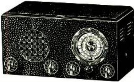
A powerful and highly efficient receiver designed for amateur communication work. Uses 7 tubes, i.e. two 6D6, two 6C5G, one 76, one 42, and one 5Y3 as *TUNED RF amplifier, TUNED electron-coupled regenerative detector, powerful 3 stage audio amplifier with pentode output stage delivering 3 watts of power to built-in dynamic speaker, rectifier and built-in power supply. Completely self-contained.*
