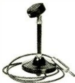
microphone setup of crystal head, stand and anti-resonant cable, and shielded plug. The microphone head is housed in a light weight aluminum shell finished in black crystalline, having a very wide open face. The unit itself is protected by a heavy monel metal screen with such opening that no sound is lost in passing through the screen. This unit is provided on a swivel head arrangement allowing the head to be placed in almost any position. The output level is high, being -55 db.
