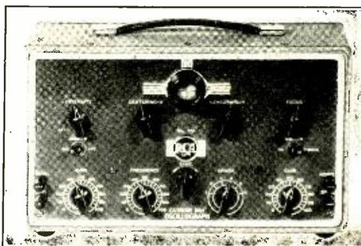
Introduced by the R.C.A. parts division is a new low-cost cathode ray oscillograph. The introduction of this new oscillograph, with a one-inch screen that meets every requirement and more of the serviceman and amateur, places this valuable instrument within the reach of additional thousands of service engineers and amateurs at half the cost of the larger, more
