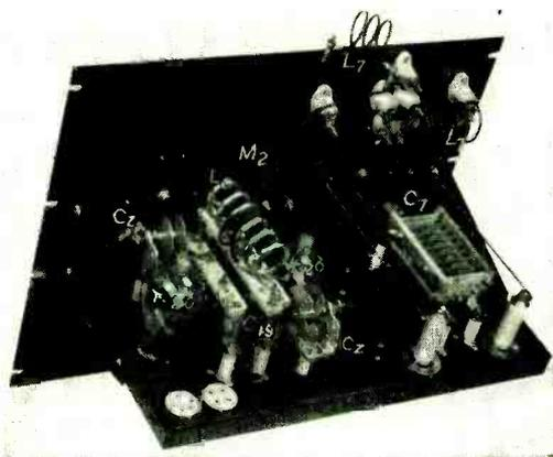
Figure 3. The push-pull T-20 final amplifier.
