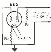
One of the magic-eye indicator tubes, 6E5, 6G5, etc., will make a very pretty little front-of-the-panel time delay indicator. The hookup of the arrangement is shown in the accompanying circuit diagram. Very simple, isn't it? Nothing but the tube and two  $\frac{1}{2}$ -watt resistors are required in addition to the regular plate and filament supplies in the rig.
