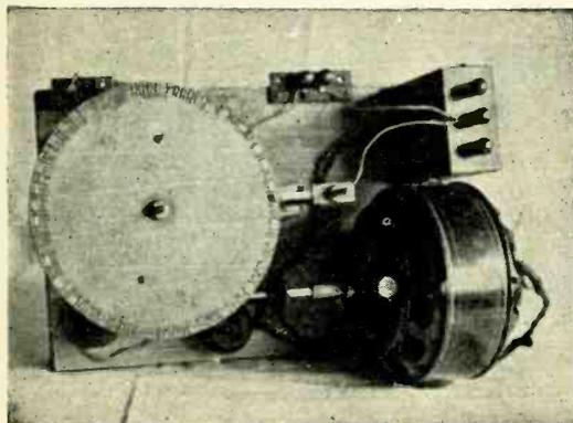
The automatic telegraphy device in use at VK2NO, for 56-Mc. long-distance test transmissions. It is made up from a fan motor and a double-reduction worm drive. The disc is of three-ply with saw cuts and interleaved copper foil to make up the Morse code characters. It sends "CQ FIVE DX DE VK2NO" at 12 words per minute.
