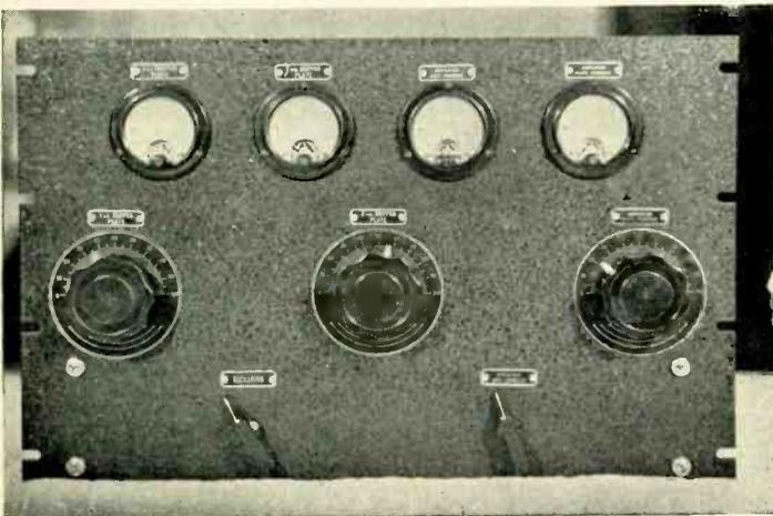
• The transmitter is built on one standard rack and panel unit. Front view of the rig is shown here.
