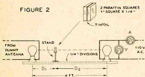
stand from thin sheet metal to hold the wax-and-tinfoil square. This stand should be of such a height that the centers of the two lamps or sets of lamps are lined up with the center of the square, figure 2.
