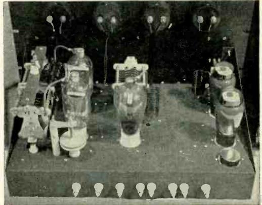
Back view shows layout of the parts in the 10-meter transmitter.
