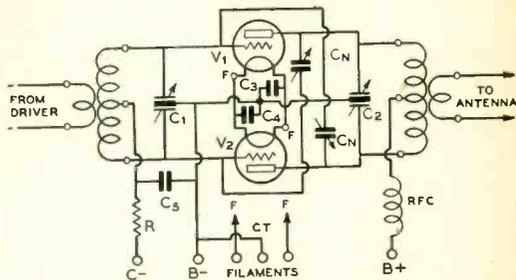
**C<sub>1</sub>**—100  $\mu$ fd. per section, 1000-volt spacing
