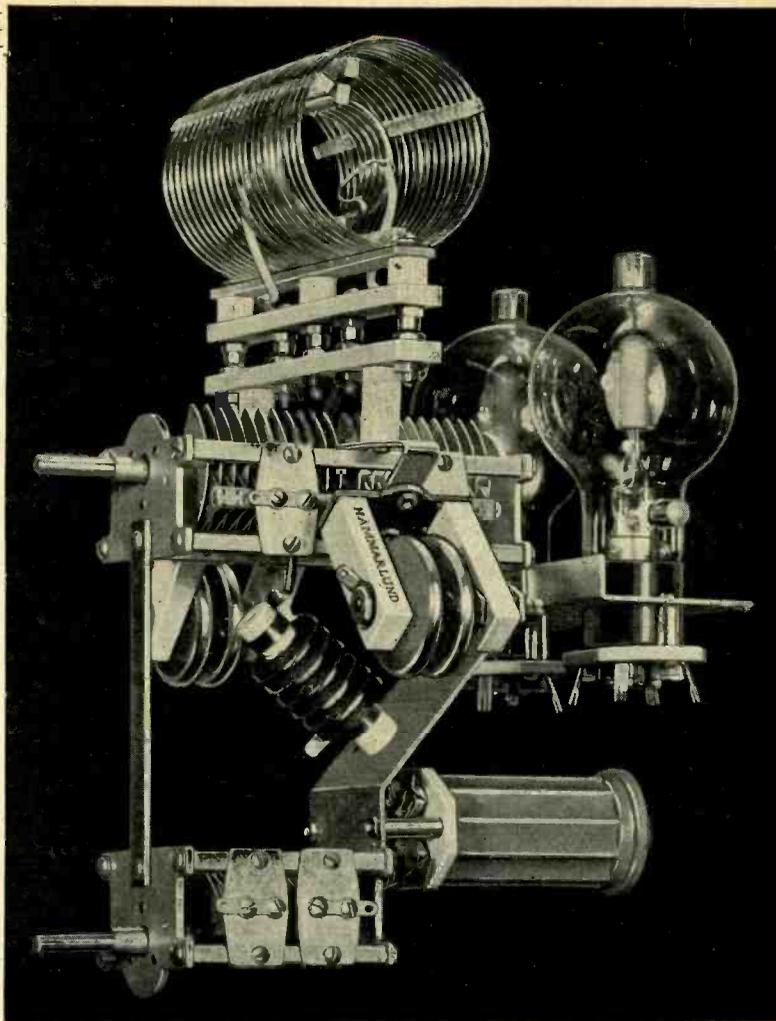
**H**AMMARLUND'S new "foundation kits" are designed to make it easier for the amateur to build neat, efficient, compact apparatus. The 300-watt push pull R.F. amplifier, illustrated, can be built in less than 20 minutes. The only tools necessary are a screwdriver and soldering iron.
