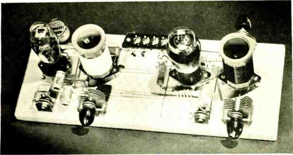
Top view of the Newcomer's transmitter showing the simplified layout. One of the 80-meter coils is shown in the oscillator and the 40-meter coil is shown in the amplifier. The neutralizing condenser is mounted behind the amplifier tank coil.
