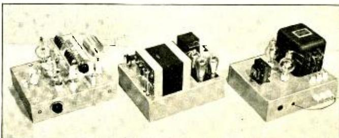
THE "BI-PUSH" EXCITER is still the most outstanding exciter brought out in the last two years. It has 40 watts output on any band, and hams throughout the world are using them. The originator, W. W. Smith, first described the Bi-Push in "Radio" for April 1937.
