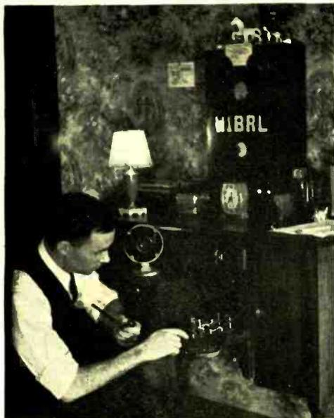
WIBRL the station of Wink Wight, taken by the OM. 27 watts input, crystal controlled, fone and c.w. on 56.096 Mc. The receiver is a resistance-coupled superhet.
