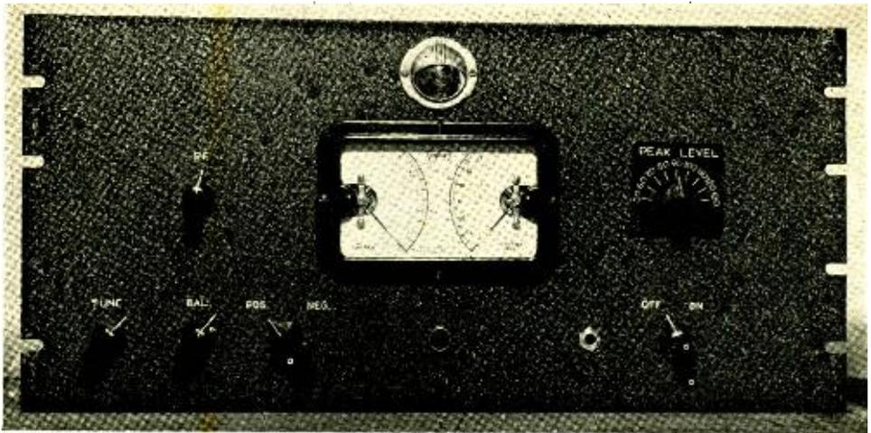
Figure Panel view of the rack-mounting type modulation indicator.
