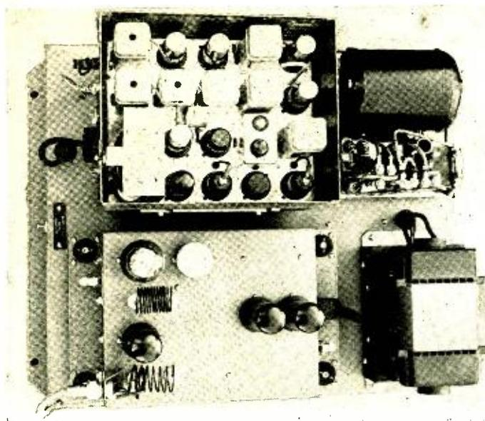
A top-of-chassis view of one of the complete units with the various covers removed. The RCA receiver with its associated power supply can be seen along the top and the four-tube transmitter, mounted upon shock insulators, with its dynamotor can be seen below.
