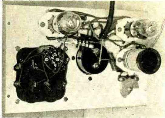
A 3-30- $\mu$ fd. mica trimmer condenser directly across the coil inside of the coil form allows this circuit to be tuned to resonance (40 meters for the above coils). It should be trimmed to drive the next doubler stage hardest in the middle of the desired range of frequencies. The unit shown is to drive a 6L6G doubler which drives a 35-T buffer which in turn excites a pair of T200 tubes in a plate-modulated rig.
