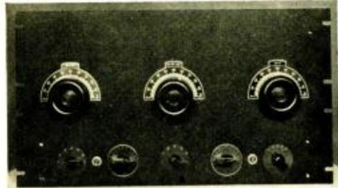
Front view of the bandswitching exciter mounted on a standard rack panel. The controls along the bottom of the chassis are: crystal selector switch, 6A6 doubler plate condenser, exciter bandswitch, final grid excitation control and final plate bandswitch.
