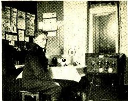
LA4K, Lorenskog, Norway. The transmitter uses an RK-20A in the final with 100 watts input on c.w. Operator is a policeman and 34 years of age.
