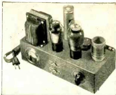
mobile or emergency transmitter. Metal tubes are supplied with the d.c. portable because of their greater ability to withstand hard usage as compared to the glass ones used with the a.c.-operated unit.
