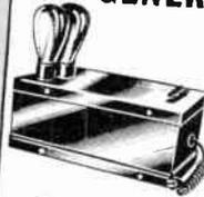
**Model 1.** In metal case 5" x 7" x 12" with binding post terminals. Delivers 500 v. pure d.c. at 150 ma. Also 7.5 volts c.t. at 5 amps. for filaments. Heavy duty transformer and filters. Operates on 115 v., 50-60 cycles a.c. Requires 2 type 81 rectifiers.
