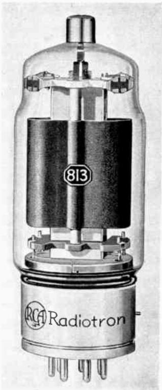
When operating as a conventional unmodulated c.w. amplifier, it is capable of giving an output of 260 watts with a driving power of 0.5 watt. A power gain of over 500, and yet the tube is operating at an efficiency of over 72 per cent. This represents a really worth-while improvement
