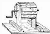
Suggested method of making string reel from old magnet wire spool with slats nailed on it. This assembly is mounted in improvised bearings with a winding crank to turn it.
