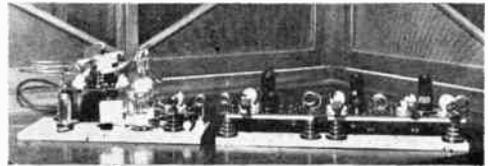
The 5-meter rig at J3FJ, Osaka, Japan, using a pair of 100TH's in the final.
