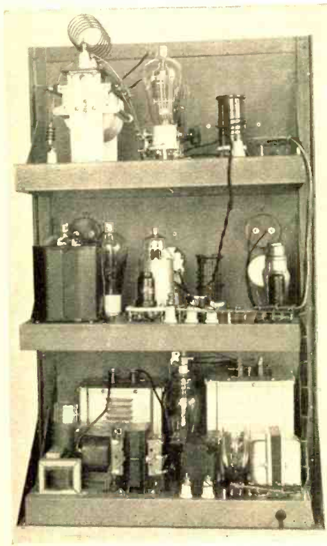
Figure 2. Back view of the T20 10-160-meter phone. The final amplifier is on the top deck, the excite- and speech stages on the second deck, and the two power supplies on the bottom deck.
