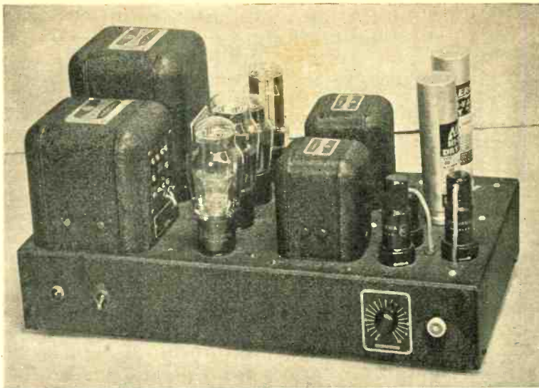
Front view of the completed amplifier. The crystal microphone plug connects to the shielded input just to the right of the gain control; automatic modulation control voltage connects to the rear of the chassis.
