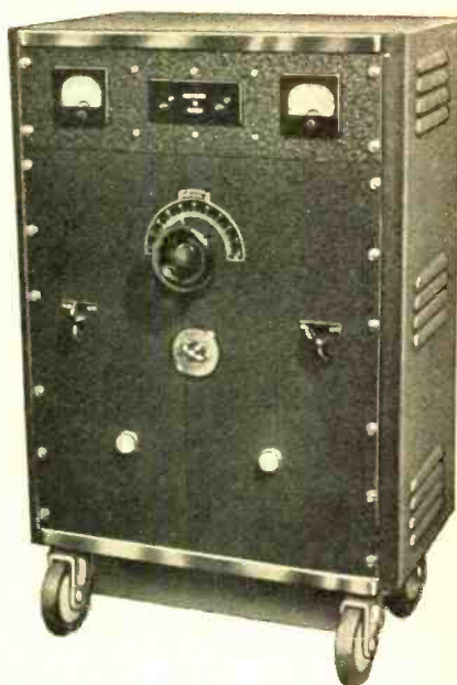
Figure 1. De Luxe 400-watt diathermy machine incorporating many safety features and worthwhile refinements. Two HF-200's are used in a push-pull Armstrong circuit.
