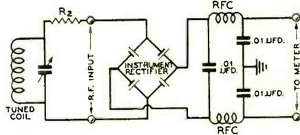
Figure 11. External circuit for measurements at high frequencies. It must, of course, be calibrated for the desired frequency of measurement.
