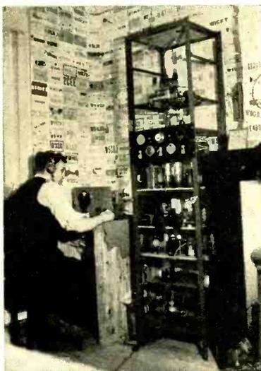
ON4HC, owned by S. Van de Wouwer, near Antwerp, Belgium. The rig uses a pair of 10's in the final amplifier with 50 watts input.
