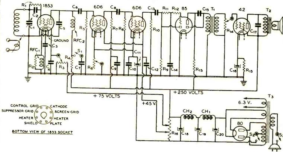
Figure 1. General wiring diagram of the improved RC superhet.
