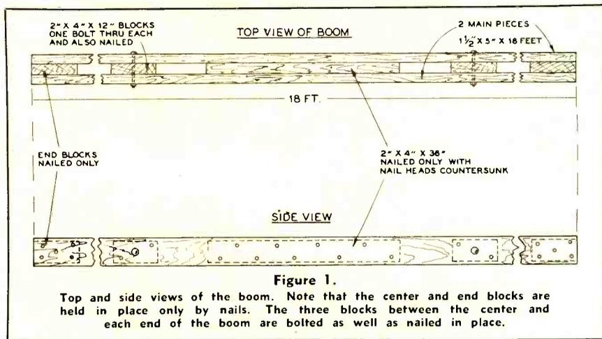
Desiring to install a new three-element 14-Mc. array that would be easy to rotate and easy to adjust, the writer spent several sleepless nights before coming up with what he believes to be a new idea in rotatable antenna construction. Since rotatable antennas of the close-spaced variety are becoming increasingly popular among the amateur fraternity, the following constructional data should be of some interest.
