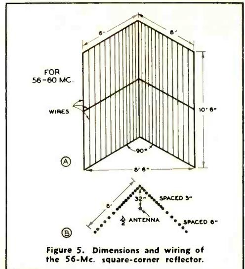
Figure 5. Dimensions and wiring of the 56-Mc. square-corner reflector.
