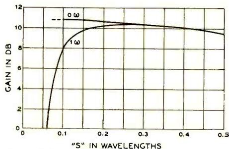
Figure 3. Variation of gain with a square-corner reflector as a function of the antenna-to-corner spacing, S.
