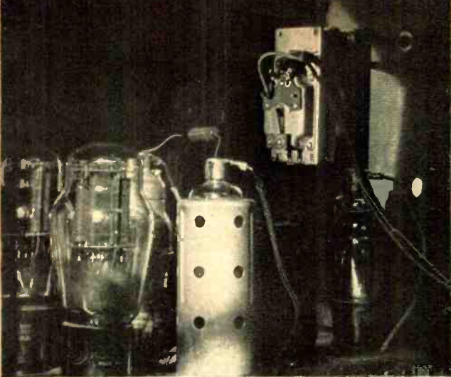
Rear view of the speech amplifier deck showing a portion of the line amplifier and the reversible a.c. motor that drives the e.c. dial.
