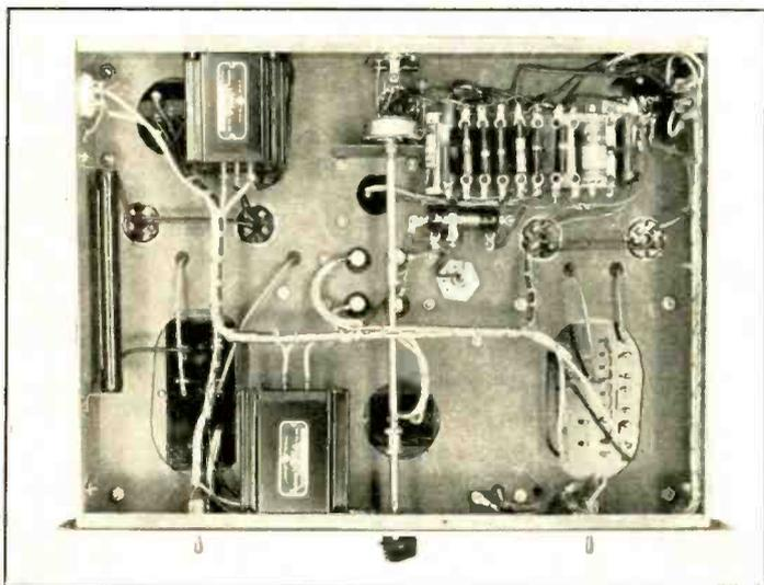
Under-chassis view of the speech amplifier, modulator, and main power supply deck. The speech amplifier components are arranged along the extreme rear of the chassis. Note the use of a large mounting bracket for the volume control and the low-level input stages of the speech amplifier.
