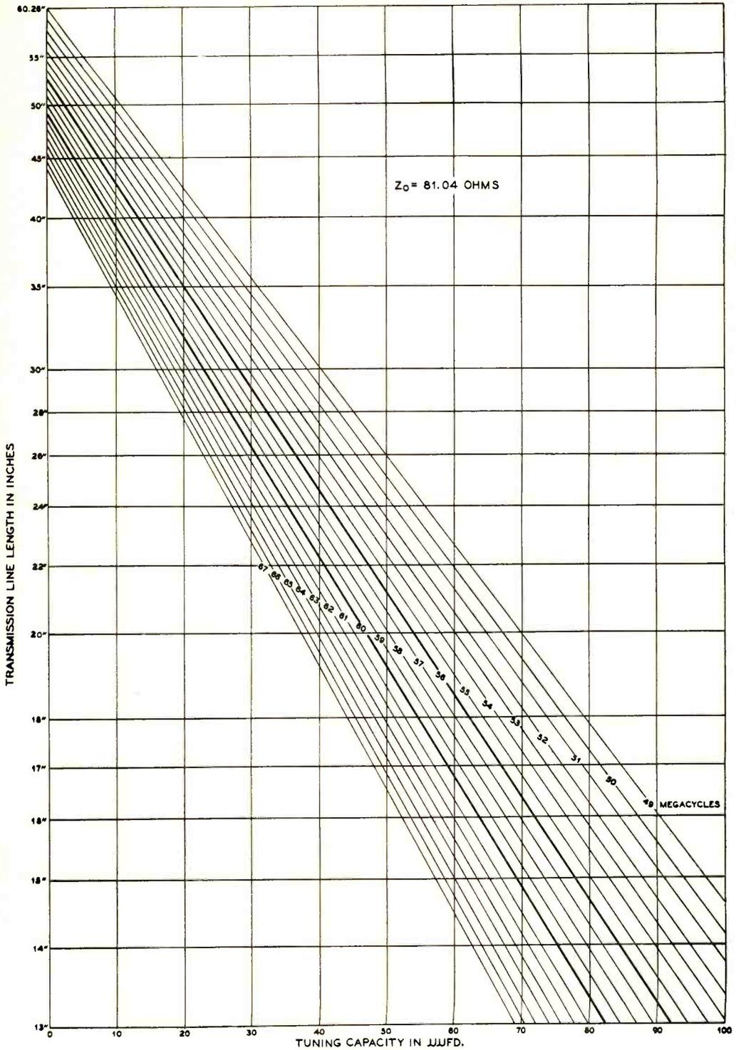
Figure 1. Chart showing capacity necessary to resonate shortened lines of 81.04 ohm surge impedance. See text for method of converting this chart to other frequencies and surge impedances.
