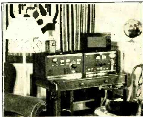
Figure 1. The modulation monitor shown in its natural habitat on the operating table to the right of the receiver. It is shown mounted in a cabinet matching that of the receiver, with a row of indicator lights for the remotely controlled transmitter below it.
