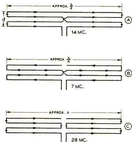
Figure 2. Arrangements of 4-wire doublet and current distributions for operation on 3 bands.
