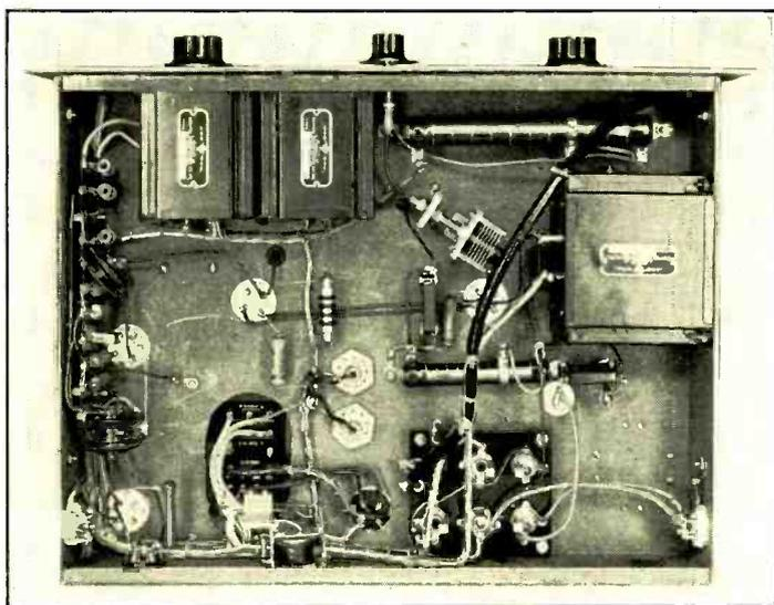
Bottom view of the r.f. section chassis. The grid condenser for the T-55 stage has been mounted at an angle and more close to the grid of the tube in order to clear the swinging choke. The condenser is rotated by means of a flexible shaft. Note the bakelite terminal board with the five jacks mounted upon it for metering the various circuits.
