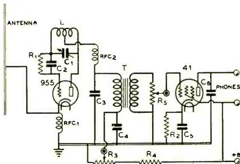
Figure 3. The 112-Mc. receiver circuit used by Kay Sheffer, W9CQV, showing the unusual method of cathode antenna coupling. Note that the r.f. section is mounted upon a piece of lucite.
