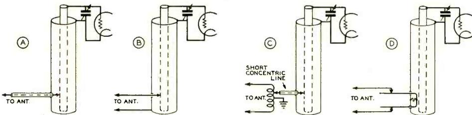
**Figure 6.** (A) coupling a concentric line feeder to a concentric line resonant circuit. (B) unbalanced method of coupling two wire line into a concentric line circuit. (C) balanced-to-unbalanced method of coupling a two wire line to a concentric line resonant circuit. (D) balanced loop method of obtaining good coupling from two wire line to a concentric line circuit.
