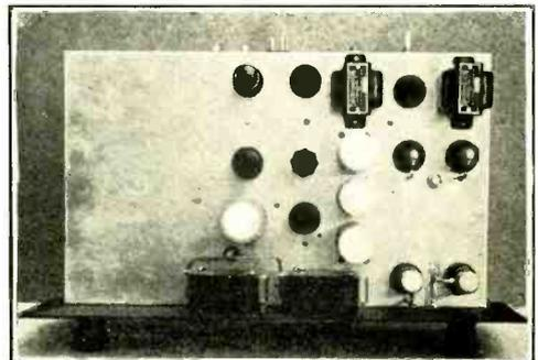
Figure 4. Looking down upon the chassis. The large space to the left is for possible future use as a mounting for a variable-frequency oscillator unit for transmitter control.
