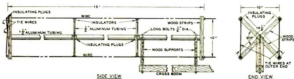
Figure 3. Experimental design of 4-wire doublet.
