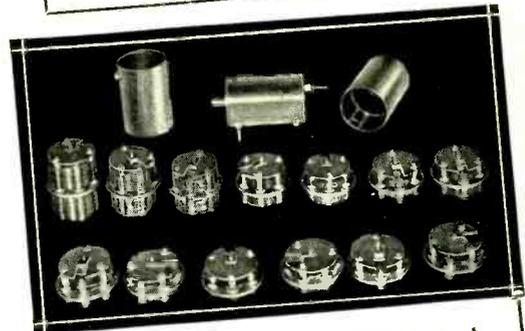
(2) A group of gold plated capacity standards of special design, made of a low temperature coefficient of expansion metal, for the largest laboratory in the world. They are mechanically and electrically . . .
