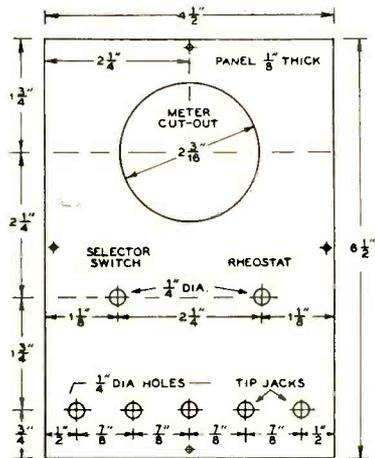
Figure 3. Front panel layout of the multi-tester.
