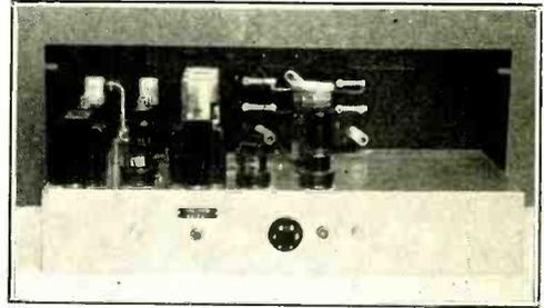
Figure 3. Rear view of the monitor-speech amplifier. The plug-in coil for 14-Mc. operation can be seen in place. The six-prong socket is for the power plug from the remote power supply.
