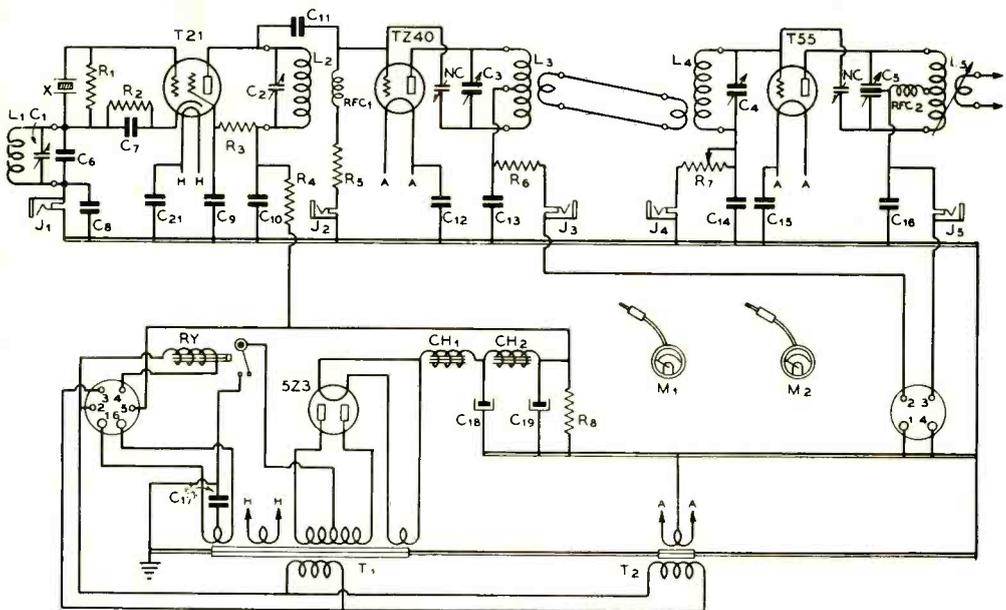
Wiring diagram of the r.f. section and the low voltage power supply.
