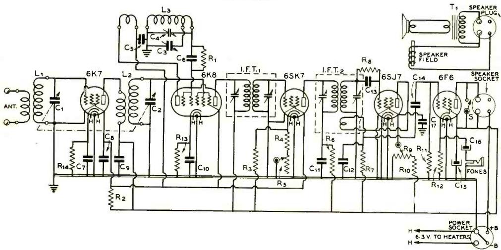
General wiring diagram of the five-tube super.
