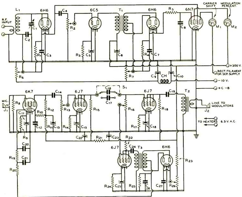
Wiring diagram of the combination modulation monitor and pre-amplifier.
