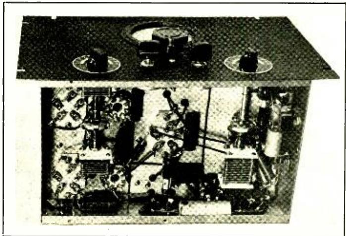
Figure 2. Most of the "works" are under the chassis. The two ganged r.f. and mixer tuning condensers are visible in this photograph, as is the oscillator bandsetting condenser.
