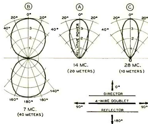
Figure 6. Measured horizontal radiation patterns of the rotary on 3 bands. The curves are plotted in terms of relative power and all curves are adjusted to the same maximum so that only the shapes of the curves are significant.
