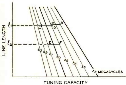
Figure 3. Exaggerated chart similar to figure 1, to illustrate method of tracking oscillator by shortening line, as described in text.
