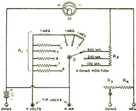
Figure 1. Schematic of the multi-tester.
