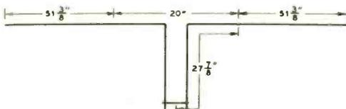
Figure 2. Final optimum lengths for the 112-Mc. extended double zepp.
