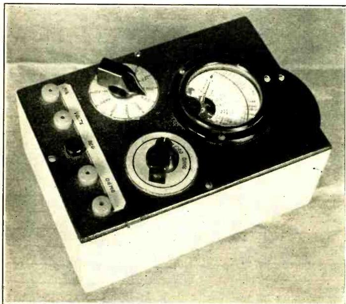
The completed multi-tester mounted in its cabinet. The panel is made of tempered presdwood and the box itself is of pine, lacquered to give a smooth durable finish. This type of mounting makes for easy portability.
