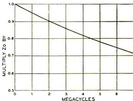
Figure 4. Chart showing constants by which mixer line surge impedance can be multiplied in order to obtain oscillator line surge impedance for tracking with lines of the same length.
