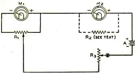
Figure 2. Current shunt calibrating circuit.
