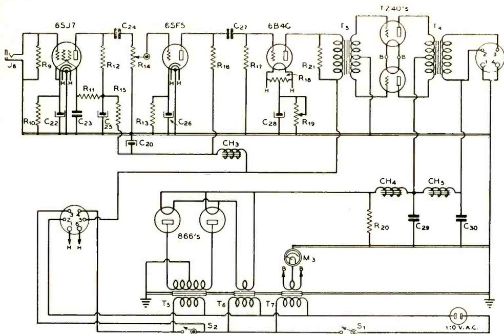
Schematic of the speech, modulator, and the high voltage power supply.
