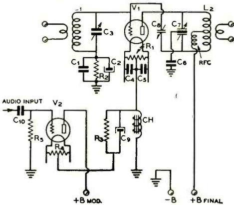
Figure 1. Wiring diagram of a single-ended r.f. amplifier being modulated by a triode parallel cathode modulator. R<sub>3</sub>, by-passed by C<sub>6</sub>, plus the drop across the choke CH furnishes the bias for the modulator tube V<sub>2</sub>.
