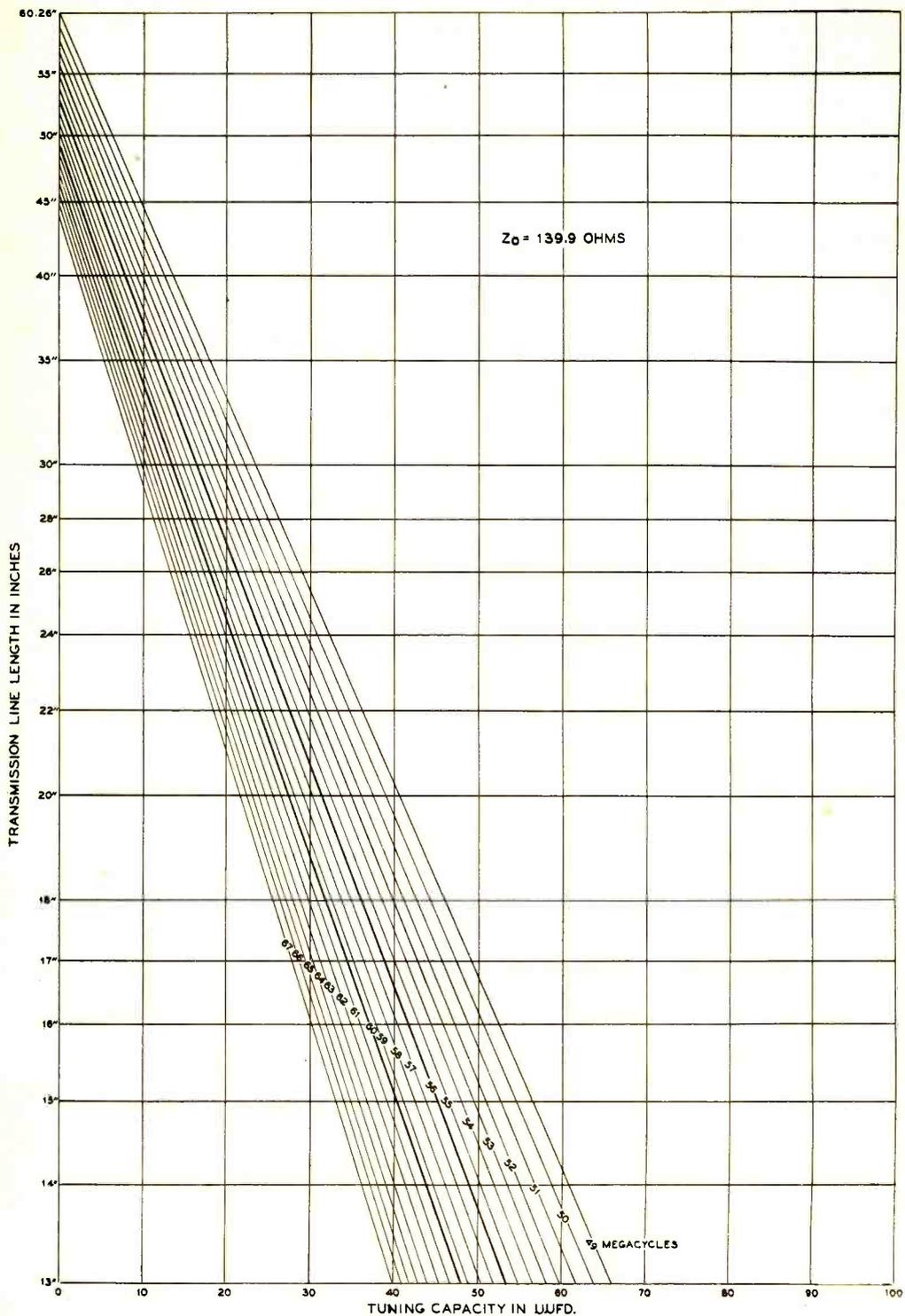
Figure 2. Chart showing capacity necessary to resonate shortened lines of 139.9 ohm surge impedance.
