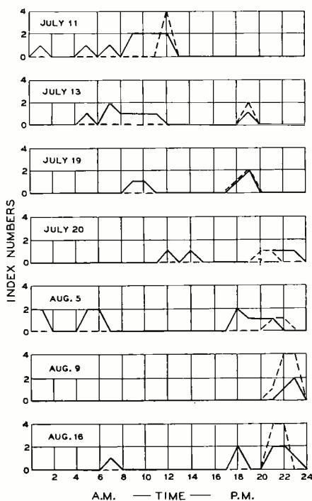
Figure 3. Hourly comparisons of sporadic-E-layer reflections observed at Washington (solid lines) with long-distance 56-megacycle reception (dashed lines), July 11 through August 16, 1937, for days of automatic observations only.
