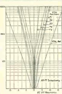
**Selectivity is variable in six steps. Curves show degree of selectivity for each step. Note that step #6 has a bandwidth at "two times down" of less than 100 cycles!**
