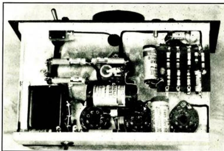
There is plenty of space under the chassis for all components. The multiplier resistors are all located on the terminal plate seen at the upper right; a cabled set of leads goes through the chassis from the terminal strip to the range switch above deck. Note the bias cell and holder, which is supported by having one of its terminals soldered directly to the grid connection on the 6SQ7 socket.
