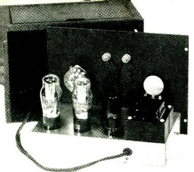
The v.t.v.m. removed from its cabinet. The power transformer, metal rectifier and the two voltage regulator tubes are in a line, from right to left across the rear of the chassis. Rubber grommets are used to insulate the meter terminals where they pass through the panel.
