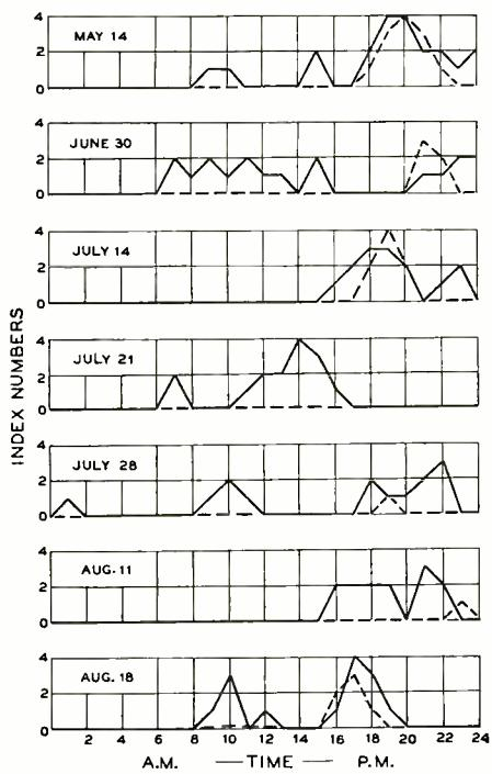
Figure 1. Hourly comparisons of sporadic-E-layer reflections observed at Washington (solid lines) with long-distance 56-megacycle reception (dashed lines) for days on which extended manual observations were made, using index numbers explained in text.
