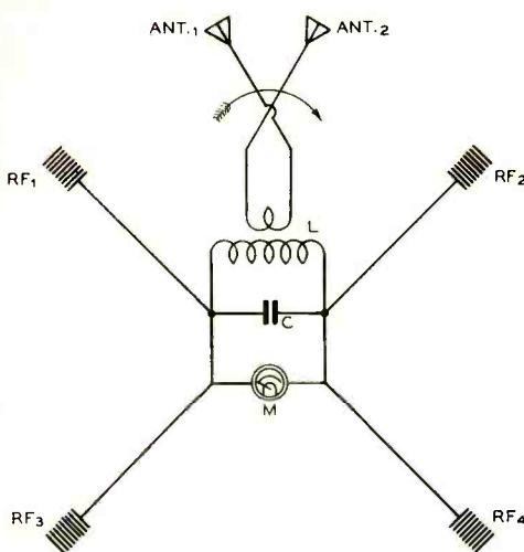
Wiring diagram of the dialogue meter.
