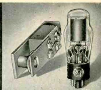
**A temperature-compensated trimmer condenser in the h-f oscillator circuit stabilizes frequency from effects of temperature changes. A voltage-regulator tube guards against frequency shifts caused by line voltage variations.**
