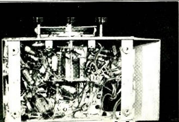
Underchassis view of the revamped receiver. The a.f. system has been left unchanged but the r.f. and i.f. channels have been completely rebuilt to the needs of FM. Full details are given in the text.
