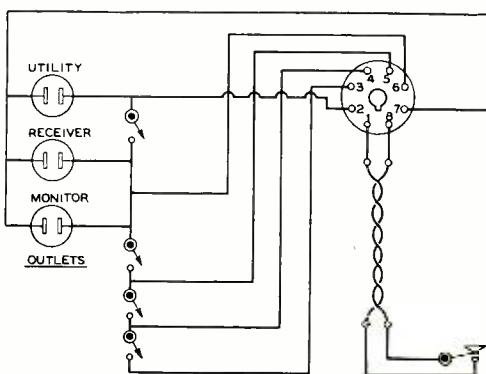
Figure 3. Schematic of the wiring at the operating position.
