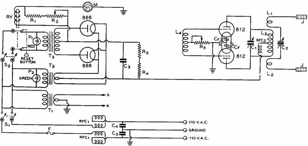
Wiring diagram of the portable diathermy machine:
