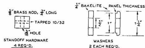
Constructional details for the plate tank condenser and the insulating washers for the pad jacks.
