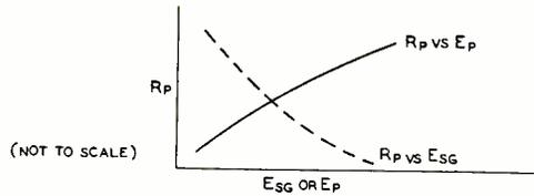
Figure 5. Variation in plate resistance plotted as a function of screen-grid voltage  $E_{sg}$  and plate voltage  $E_p$ .
