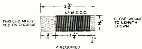
Four a.c. line chokes, made as in the above drawing, are required. All chokes are wound in the same direction on  $\frac{3}{4}$ " round wooden dowel with no. 16 d.c.c.
