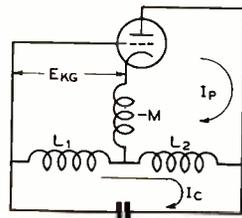
Figure 2. Hartley oscillator showing a.c. current flow and mutual inductance between portions of the tank circuit.
