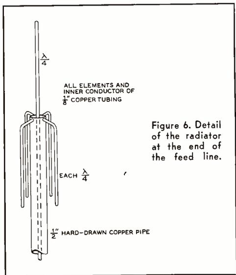
Figure 6. Detail of the radiator at the end of the feed line.
