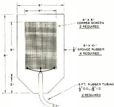
Drawing showing the method of making the diathermy pads.
