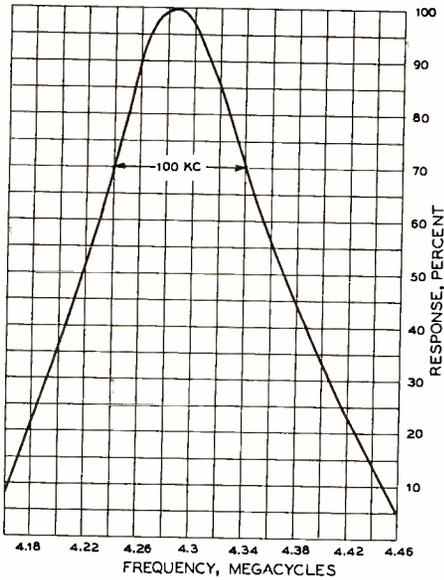
Figure 3. I.f. response characteristic of the FM converter. Output held constant at 20 microamperes in the limiter grid leak.
