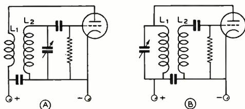
Figure 3. Ticker feedback oscillator. (A) Plate tickler version, (B) grid tickler arrangement.
