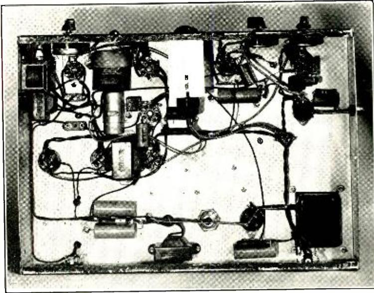
Under chassis view of the 15 watt compression amplifier. Observe that the small chokes  $CH_1$  and  $CH_2$  are mounted as far as possible from the power transformer.
