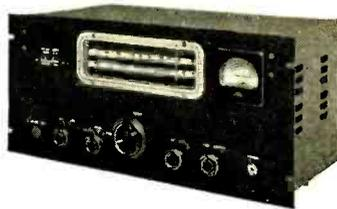
The S-31 provides a dual i.f. system, the 4.3 mc. FM channel utilizing 1852 and 1853 tubes in its two 4.3-Mc. stages, a 6SJ7 limiter and 6H6 discriminator. The 455-kc. AM channel includes a single 6SK7 with special band-pass input circuit, and a 6SR7 which serves as detector and a.v.c. and its triode section as the output stage for both AM and FM channels and also for phono. A 6SK7 t.r.f. stage and 6SA7 converter provide the r.f. input to both channels.
