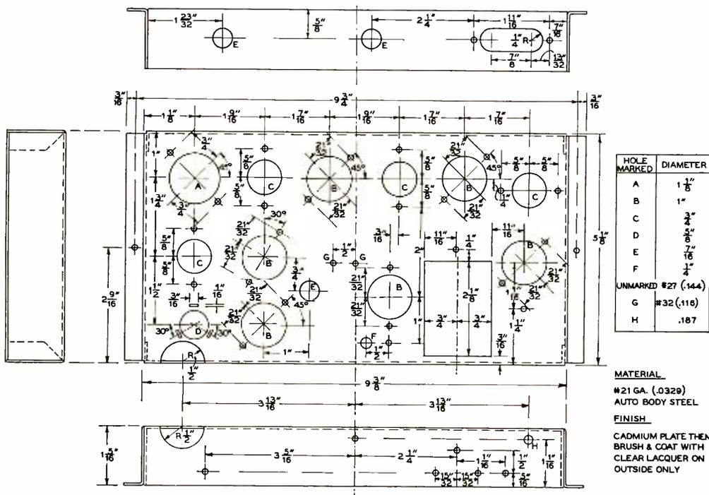
FIGURE 9. LAYOUT DIAGRAMS FOR THE FRONT PANEL AND THE TUNING CONDENSER MOUNTING BRACKET.
