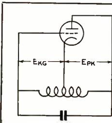
Figure 1. A.c. details of a Hartley oscillator.
