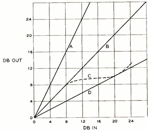
Figure 1. Illustrating various input-output level amplifier characteristics. Curve B is that of a normal amplifier. Curve C is that of the compression amplifier of figure 2.
