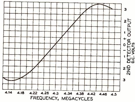
Figure 4. Second detector (discriminator) characteristics of the FM converter. The curve was taken with 2 volts input to the limiter grid.
