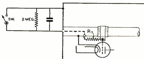
Figure 4. Method of altering the grid leak resistance of the oscillator for using the unit for a transceiver.  $R_1$  is adjusted to the proper value to make the tube draw its rated plate current when feeding the antenna as a transmitter. With the switch opened the tube operates in the conventional manner as a superregenerator.
