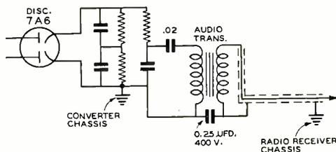
Figure 7. An optional method for coupling the audio output of the converter into the audio power amplifier.
