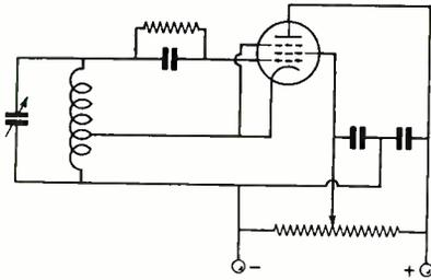
Figure 4. The Dow or electron-coupled oscillator.
