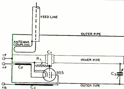
Figure 3. Semi-schematic wiring diagram of the 400-Mc. receiver. The grid-coupling,  $C_1$  filament by-pass,  $C_F$ , and plate by-pass condensers,  $C_2$  are described in the text. The grid leak  $R_1$  is 2.0 megohms.
