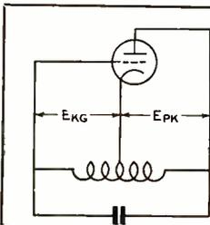
Figure 1. A.c. details of a Hartley oscillator.
