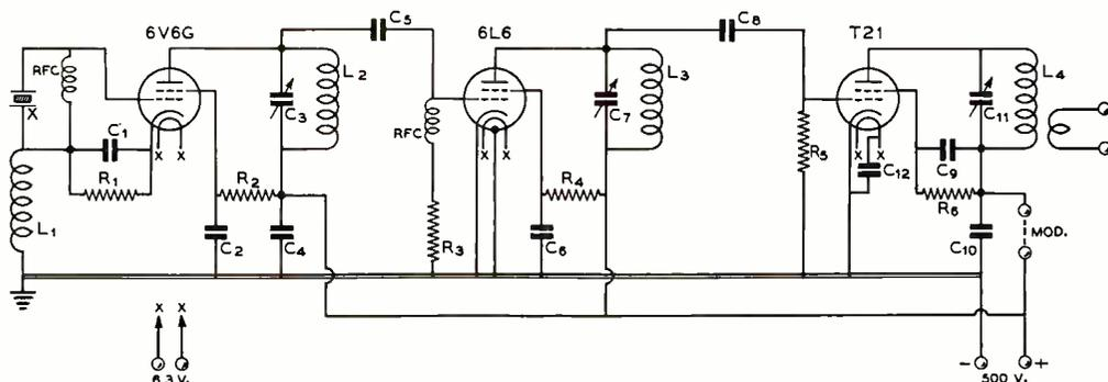
Wiring Diagram of Modified Rothman 56 Mc. Transmitter
