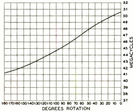
Figure 10. Frequency vs. dial reading calibration curve for the converter.
