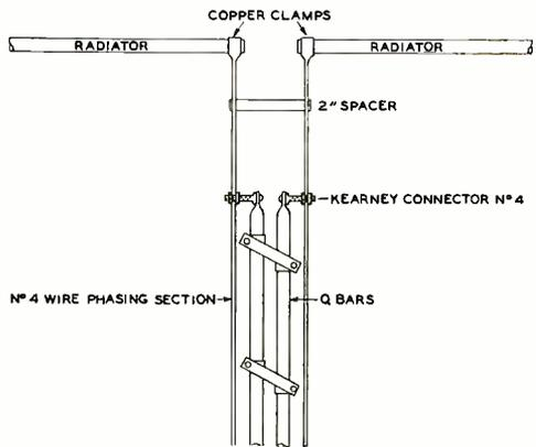
In the particular case of the array described, the standing wave ratio worked out to be 12-to-1, which meant (since a 500-ohm line was being used) that the impedance to be matched was about 40 ohms. The geometric mean between 500 and 40 is 142. Hence the quarter-wave section should have a characteristic impedance of 142 ohms. This value of impedance was obtained by means of a Q section composed of standard 1/2-inch tubing spaced 0.8-inch center to center and 4 feet 1/4 inch long.
