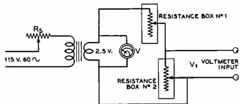
Figure 5. Circuit for calibrating the lower ranges.  $R_s$  is adjusted for a reading of 2 volts on  $V_1$ .  $V_1$  will then be equal to the resistance across the terminals of box 2 times .001. The sum of the resistances of the two boxes should be 2000 ohms at all times.
