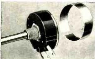
**STANDARD:** Wall type resistor hugs inner circumference of black moulded bakelite case. Exclusive non-rubbing contact band for quiet, smooth rotation and long life. 1 3/8" diameter x 9/16" deep. Available single, twin, or triple, plain or tapped with one or two taps . . . with S.P.S.T., D.P.S.T., or S.P.D.T. Metal shaft extends 3 3/8" from case
