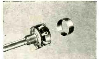
**ELF:** Small, but also features the long, straight resistor strip. Available plain or tapped with S.P.S.T. Switch . . . with or without dummy lug. Switch rated 2 Amps. 125 V. Underwriter's approved. Bakelite case 57/64" diameter, 17/32 deep (less switch) 25/32" deep with switch.
