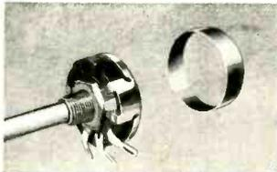
**MIDGET:** Companion to "Standard" . . . small size but large control efficiency. Available single, dual or triple . . . plain or one, two or three taps . . . with S.P.S.T., S.P.D.T., or D.P.S.T. Moulded bakelite case, 1 1/8" diameter, 1/4" metal shaft 3 3/8" long.
