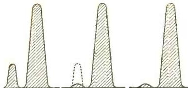
With selectivity switch in XTAL sharp position identify the weaker amplitude — Tune Receiver to the weaker.
