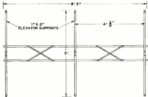
Figure 3. Detail drawing of the phasing section and the Q bars.
