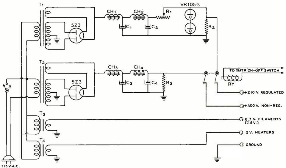
Schematic of Power Supply Unit
