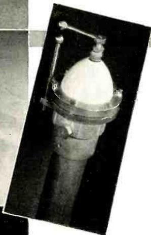
Above is illustrated an R. F. Make-Before-Break Switch for inserting and removing a meter without breaking the circuit. The R. F. Contactor uses knife-type contacts and requires no holding current. The Isolation Transformer is used to feed sampling lines and for remote metering. Shown also is a terminal and safety gap for Johnson 2 5/8 inch concentric line.
