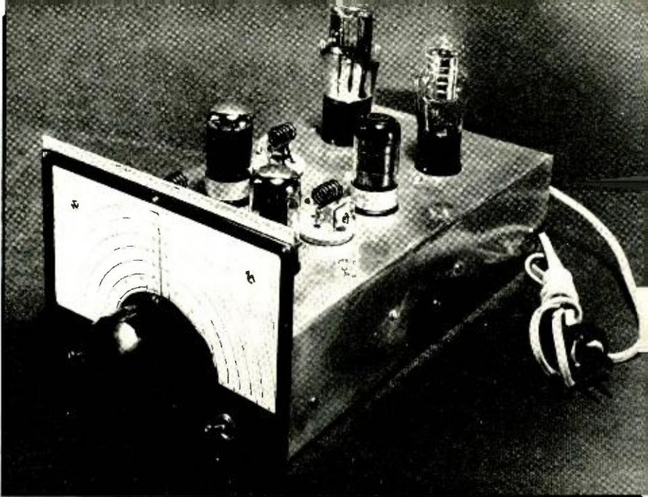
The a.c. and standby switches are mounted in holes drilled through the dial itself. From front to back—the oscillator coil and tube, the mixer tube and coil, the r.f. coil and tube, and the rectifier and regulator tubes.
