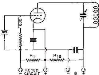
Figure 5. Method of connecting the bug to the keyed stage. The resistors  $R_{11}$  and  $R_{12}$  are also included in the main circuit diagram, but may actually be placed either in the bug unit or at the keyed stage.
