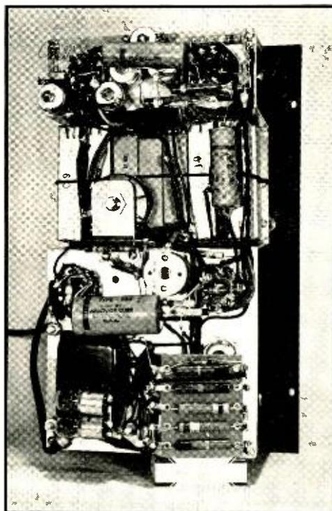
parallel several resistors until combinations are found which give the correct values. Your voltmeter will be as accurate as your attenuator resistors. When this is completed, switching from one range to another and at the same time increasing or decreasing the input voltage by a factor of 10 should produce identical meter readings. You will then know that the voltage calibration which you obtain on any one range will be reproduced on any other range with the proper factors of 10 accounted for.
