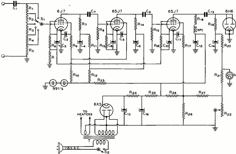
Figure 4, Wiring Diagram
