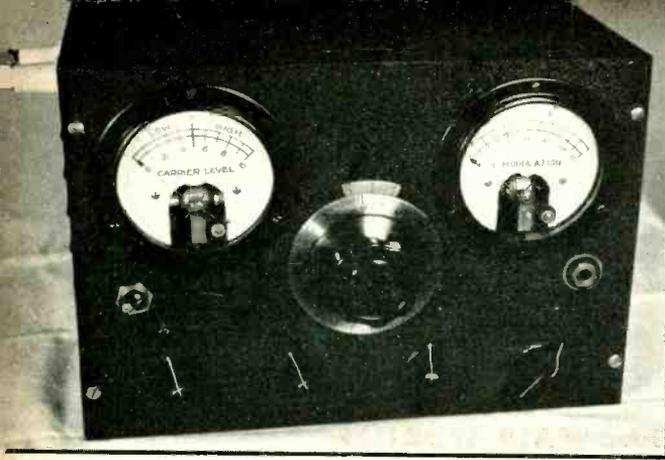
Figure 1. The completed transmitter test set. The lower controls, left to right, are: audio gain, bandswitch, degenerative feedback voltage, and a.m.c. bias. Above are the phase switch, the main tuning condenser, and the 'phone jack.
