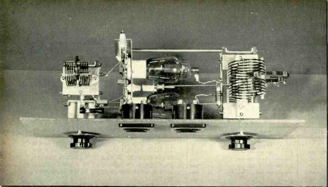
Top view of the amplifier. Only one of the plates had been removed from the neutralizing condenser when this photograph was taken. It was later found necessary to remove this remaining plate also and to replace it with a 1/2-inch machine screw. The method of mounting the various components can be clearly seen in this photograph.
