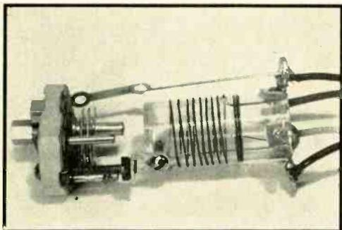
Figure 1. One of the coils used at  $L_1$  and  $L_2$  shown removed from its shield can. These coils are wound on  $\frac{1}{2}$ -inch polystyrene coil forms. The closed end of the form was drilled and tapped on the side to take a 6-32 brass screw. A small angle bracket and a 4-40 by  $1\frac{1}{2}$ -inch bolt holds the coil form to the trimmer condenser.
