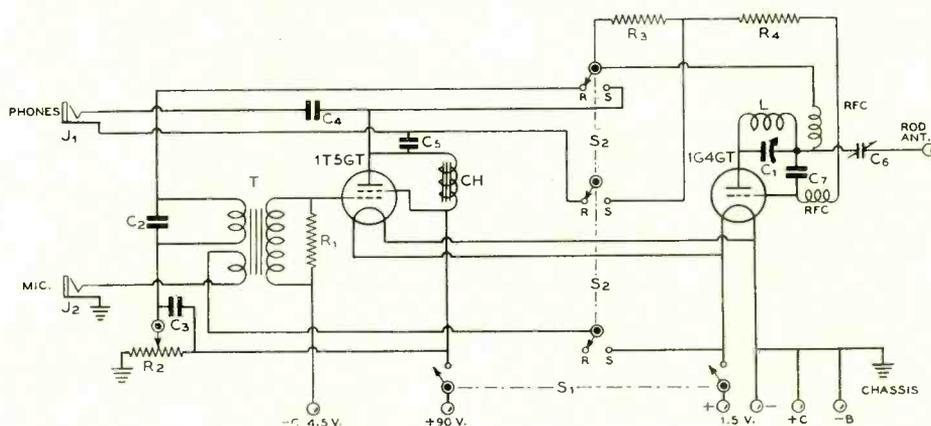
WIRING DIAGRAM OF THE SELF-CONTAINED TRANSCIEVER.
