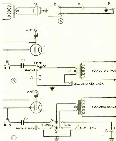
Figure 2. Three methods of obtaining a tone for i.c.w. The system of "C" is essentially the same as that of "B" except that a d.p.d.t. switch makes it unnecessary to plug the mike and key plugs in and out when changing from voice to i.c.w.
