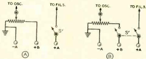
Figure 4. By using a d.p.s.t. switch instead of a s.p.s.t. as the off-on switch, there is no danger of running down the batteries by the regeneration potentiometer drain while the set is not in use.
