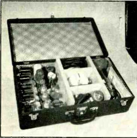
Figure 3. The accessory kit. Note how neat compartments have been built into the kit—with sockets for the coils, tubes, and crystals—so that everything will be in its place when the cover is opened at the field operating position.
