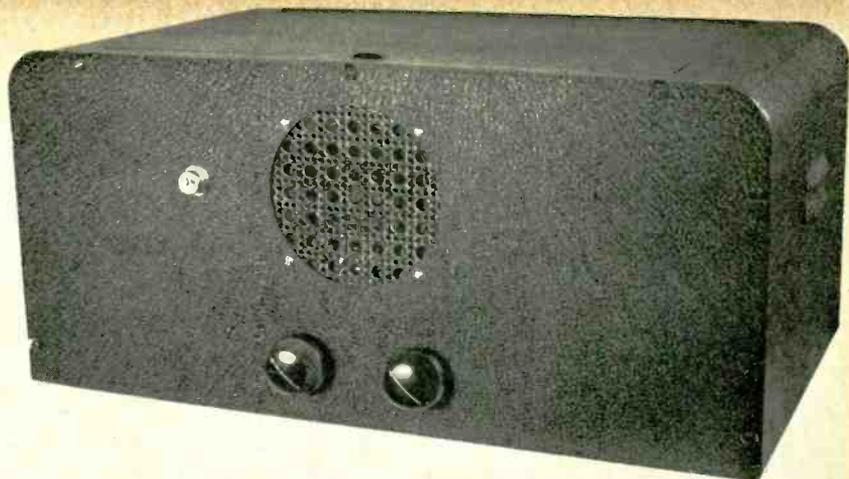
both frequencies. These three features can be listed as "musts" for such a receiver: crystal control of the h.f. oscillator, automatic volume control, and a good signal-to-noise ratio. The front end of any superhet receiver is always improved by the use of a preselector stage, so one was incorporated into the design of this superhet.
