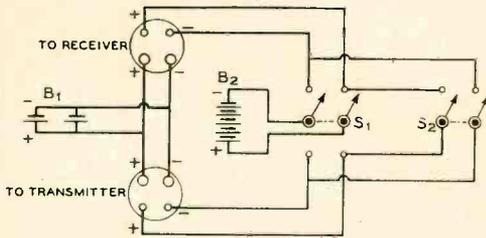
Connections inside the portable battery box.
