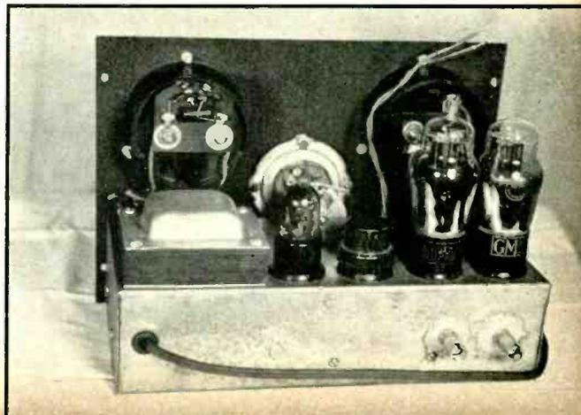
The calibration will remain accurate as long as the life of the tubes used in the gimmick, but should always be rechecked whenever any tubes, with the exception of the rectifier, are changed. When taking a reading of percentage modulation on the meter, coupling to the transmitter should always be adjusted to give deflection of the carrier level meter needle to the center or zero point on that dial. Dials for the meters can be made from fiber board or any such suitable material.
