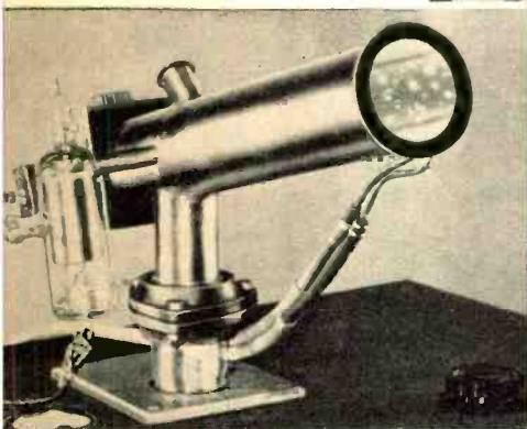
Close observation of the flow of electrons from a heated filament is made possible with this Electron Microscope. This instrument, designed and constructed in the Eimac laboratories, virtually gives a motion picture projection of the electron movement.
