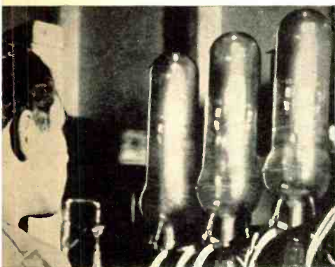
Before filaments are sealed into the triode they are placed in a temporary vacuum where they undergo their first emission test. Thus faulty filaments may be weeded out without further processing.
