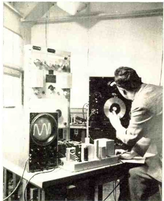
This small amplifier shown being tested with a cathode-ray oscillograph is used principally for monitoring the output of broadcast transmitters.
