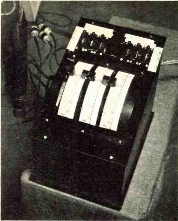
Control device used in "stereophonic" recording by which frequencies, amplitudes, and spatial relationships of sound can be altered to enhance the effect of the reproduction.
