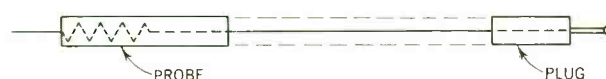
Fig. 4. In some designs the filter resistor is placed in the probe end of the shielded cable.
