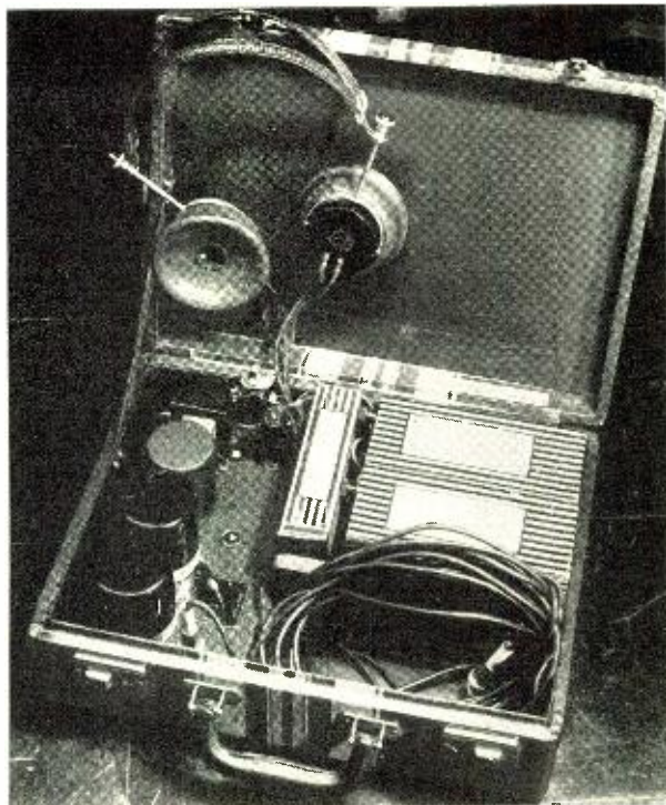
The portable, battery-operated bomb detector. It is housed in a lady's overnight case with inside dimensions of 12 \frac{1}{2} " x 9 \frac{1}{4} " x 4" deep. Any similar case will do.
