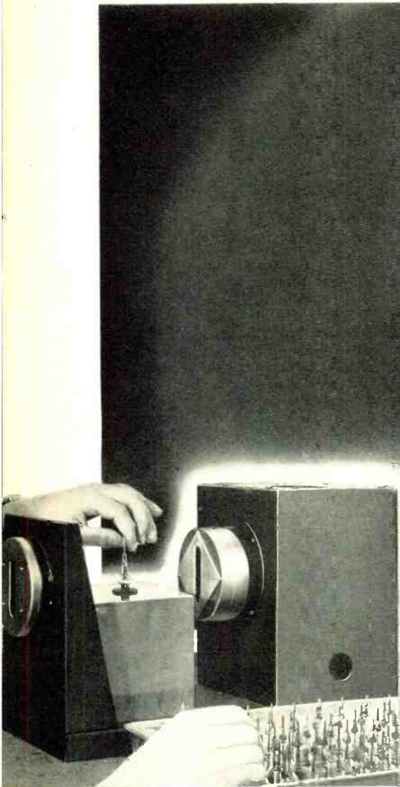
Observation of the stress points on glass bead seals around vacuum tube leads is made with this device. Close-up photo above shows the actual view of a faulty lead. Note the change in polarized light creating distorted shadows which show up stress and strain in beads. Such strain sometimes occurs where metal and glass are sealed together.
