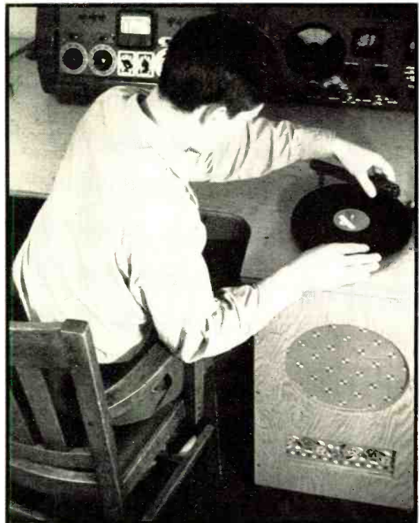
Cueing in a record. This view shows details of the bass reflex speaker inclosure, with lower port. Speaker cavity adjustment is covered in text.
