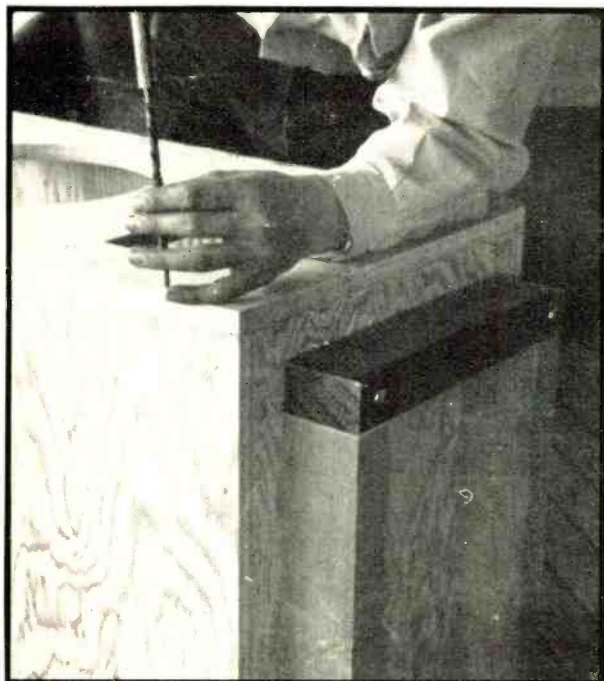
The speaker end of desk, made of \frac{3}{4} " plywood. Note heavy 2 by 3 base which leaves foot room around edges.
