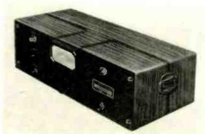
Frequency is indicated directly on front panel of meter or on separate recorder. The meter has an input impedance of 100,000 ohms or over. It will measure frequency regardless of input signal voltage variations between 1/2 and 200 volts. Stability is maintained with line voltage variations between 105 and 125 volts.
