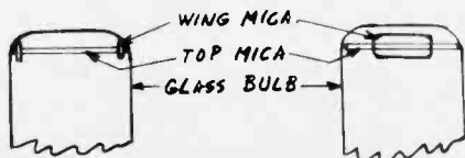
Top mica in receiving tube used as positioner and vibration cushion
