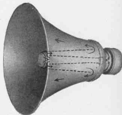
Left —MARINE SPEAKER; approved by the U. S. Coast Guard, for all emergency loudspeaker systems on ships. Re-entrant type horn. Models up to 50 watts. May be used as both speaker and microphone.
