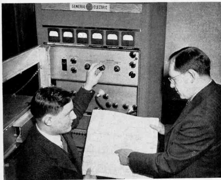
ST relay equipment, such as that shown above, will be used for setting up wireless FM networks. Such grids may be operated as public utilities.
