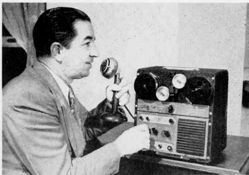
F. A. Ray, of General Electric's Electronics Dept., using new model of magnetic wire recorder being built by G.E. for armed forces. Device will take 66 minutes of recording, and same wire can be re-used 100,000 times.
