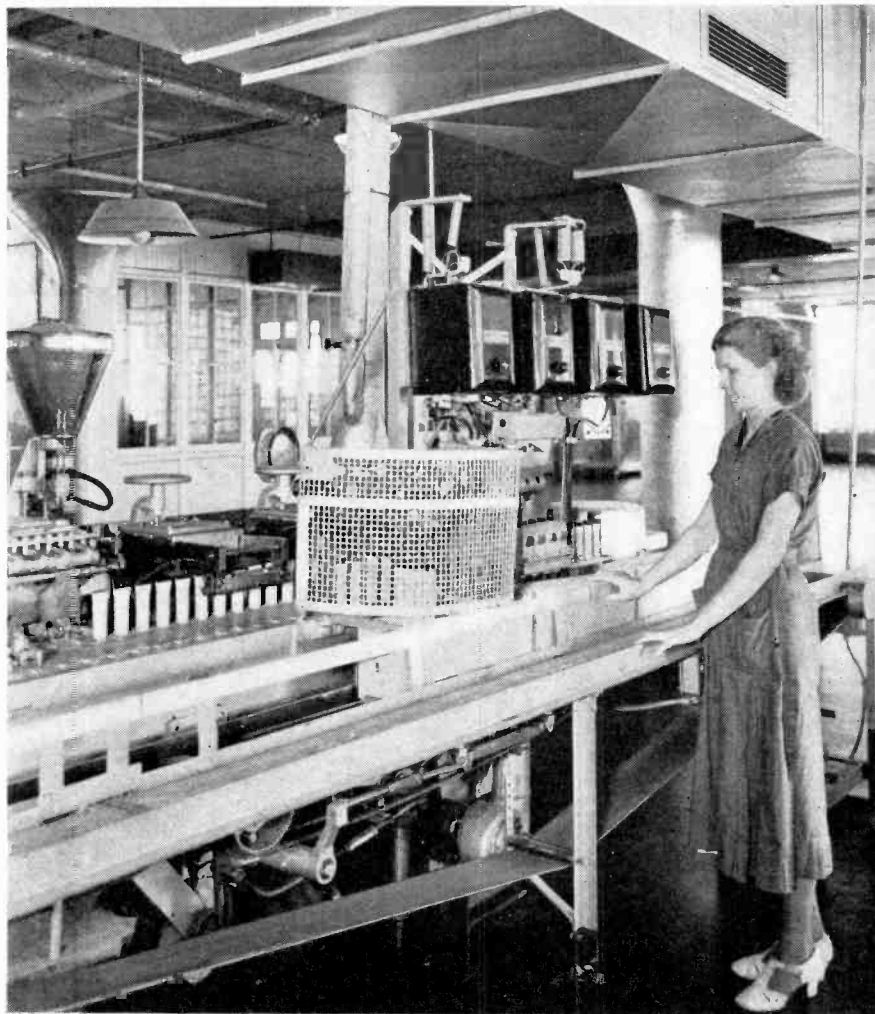
C. E. photocell relays controlling toothpaste-tube fillers in Bristol-Meyers plant
