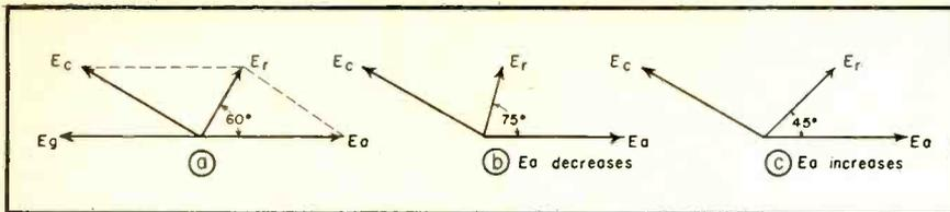
Fig. 5. Vector diagrams of plate tank voltage. See text
