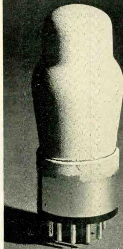
• This electrical replica of a heater-type pentode was made for use in German telephone repeaters.
