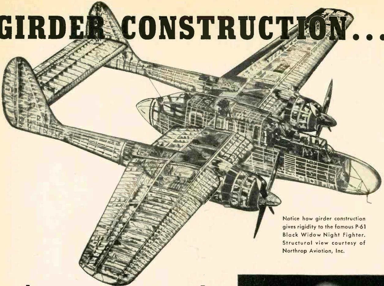
Notice how girder construction gives rigidity to the famous P-61 Black Widow Night Fighter. Structural view courtesy of Northrop Aviation, Inc.
