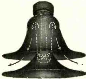
*Left*—RADIAL HORN SPEAKER; a 3½' re-entrant type horn. Projects sound over 360° area. Storm-proof. Made of RACON Acoustic Material to prevent resonant effects.
