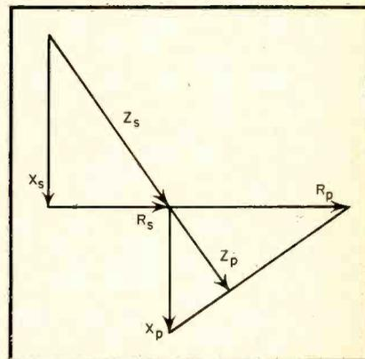
Fig. 5. Impedance vectors of R-C network tuning at oscillating frequency where  $R_s/C_s$  is not equal to  $R_p/C_p$
