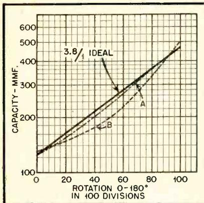
Fig. 6. Condenser capacity curves, the ideal logarithmic for a 3.8/1 range R-C oscillator, "A" a padded broadcast condenser suitable for this range, and "B" a condenser less suitable for this range
