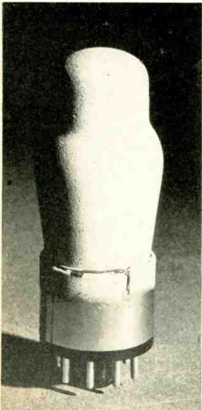
The Bradley tube, duplicate of German-made repeater, made by Western Electric for Belgian telephone systems
