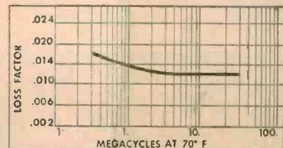
Based on Power Factor Measurements made by Boonton Radio Corp. on standard Mykroy stack.
