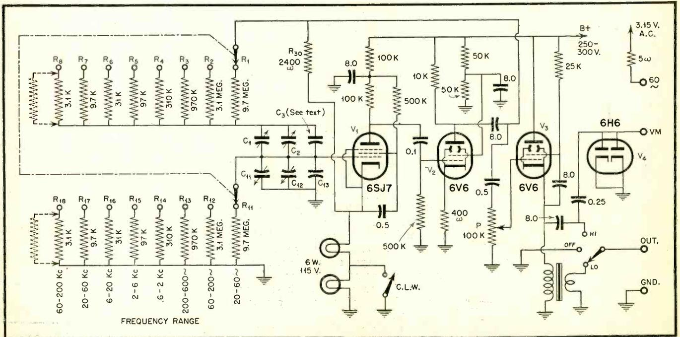
Fig. 1. Schematic of the oscillator tuned by R-C network with variable capacitors
