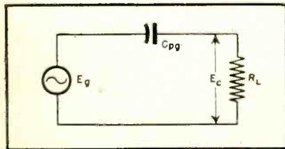
Fig. 4. Phase shift due to tube capacitance
