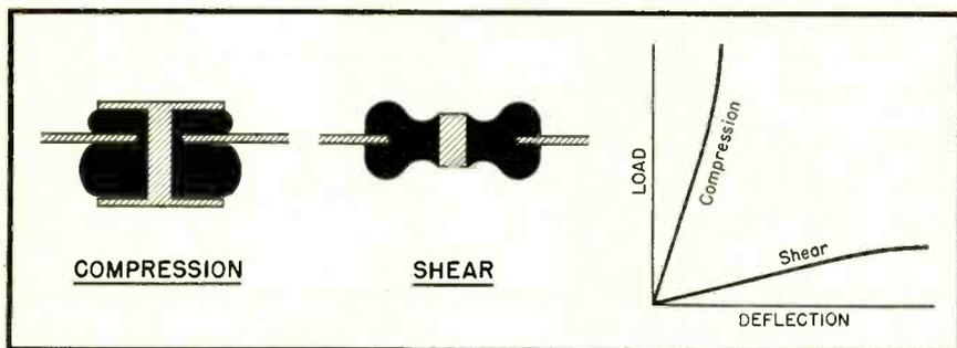
Fig. 1. Rubber shock mountings in compression and shear
