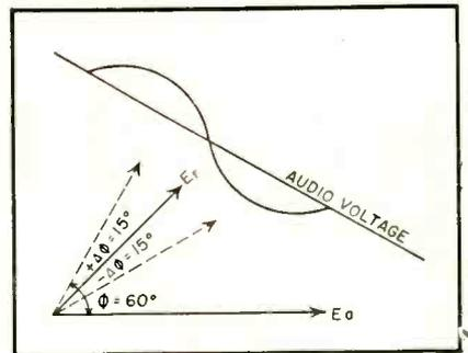
Fig. 6. Phase change is a maximum for positive and negative peaks of audio voltage
