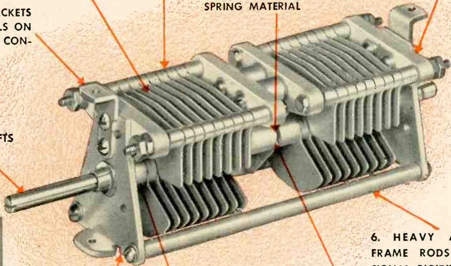
6. HEAVY ALUMINUM FRAME RODS FOR TORSIONAL RIGIDITY.
