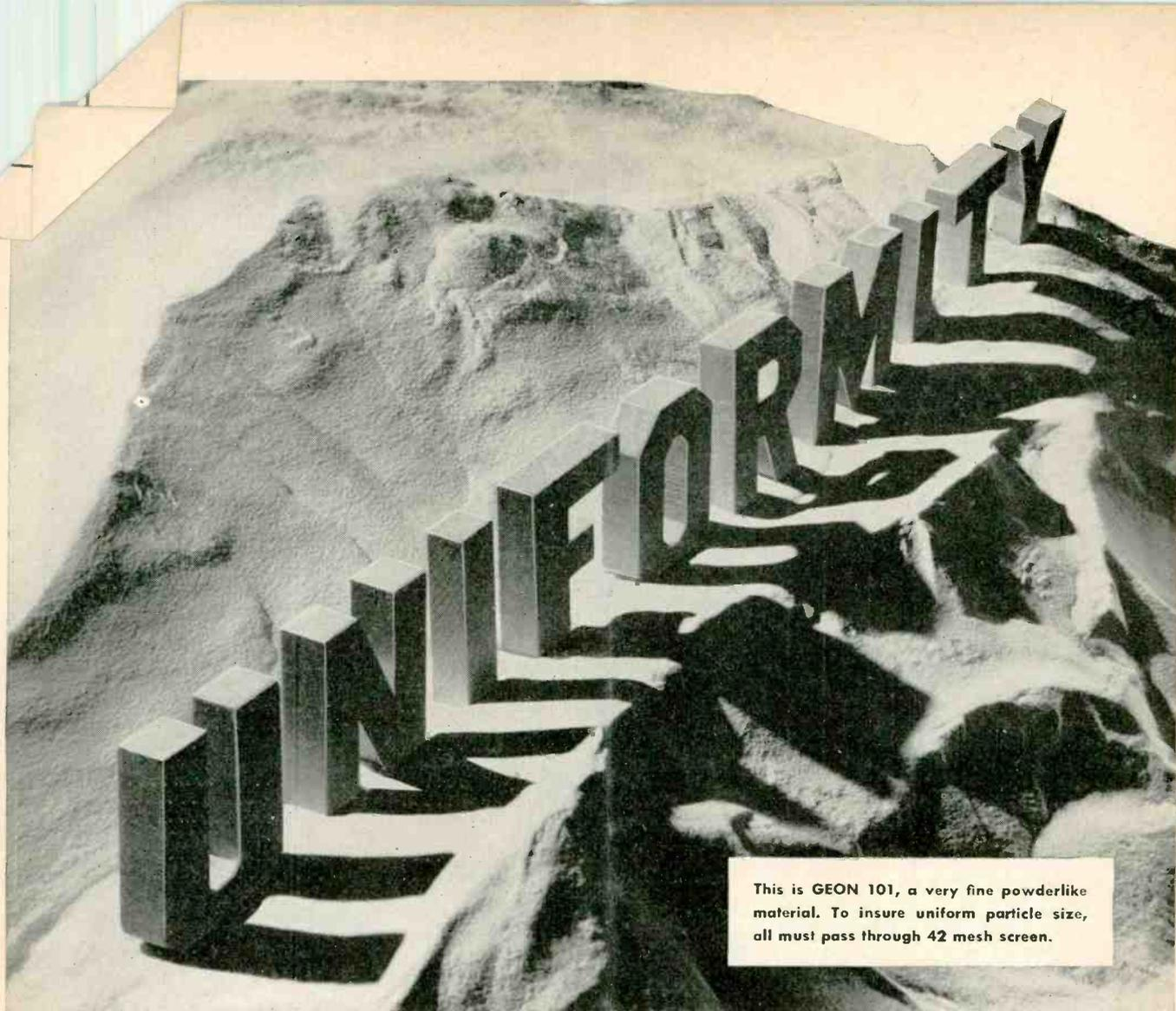
This is GEON 101, a very fine powderlike material. To insure uniform particle size, all must pass through 42 mesh screen.
