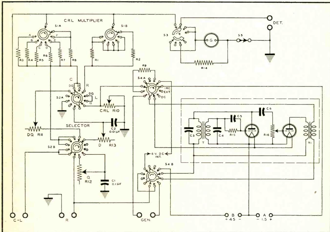
Fig. 2. Complete schematic of the CRL Impedance bridge
