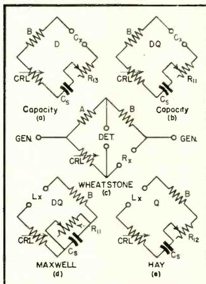
Fig. 1. Fundamental circuits used in impedance bridge
