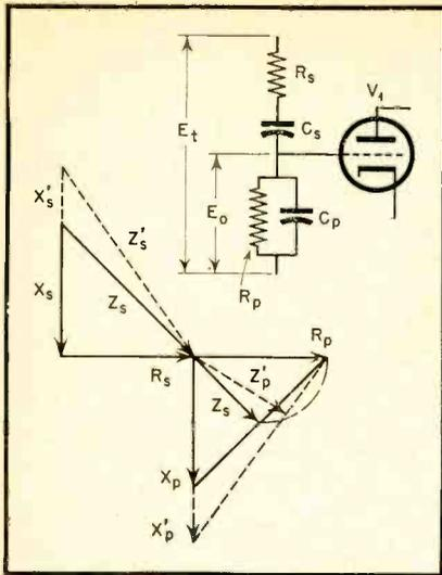
Fig. 2. Impedance vectors of R-C network,  $R_s = R_p$  and  $C_s = C_p$ . Solid lines at oscillating frequency, dotted lines at lower frequency
