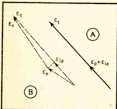
Fig. 3. Voltage vectors for Fig. 2: (a) at oscillating frequency, (b) at lower frequency
