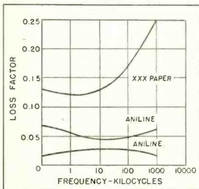
Fig. 3. Loss factor vs. frequency curves
