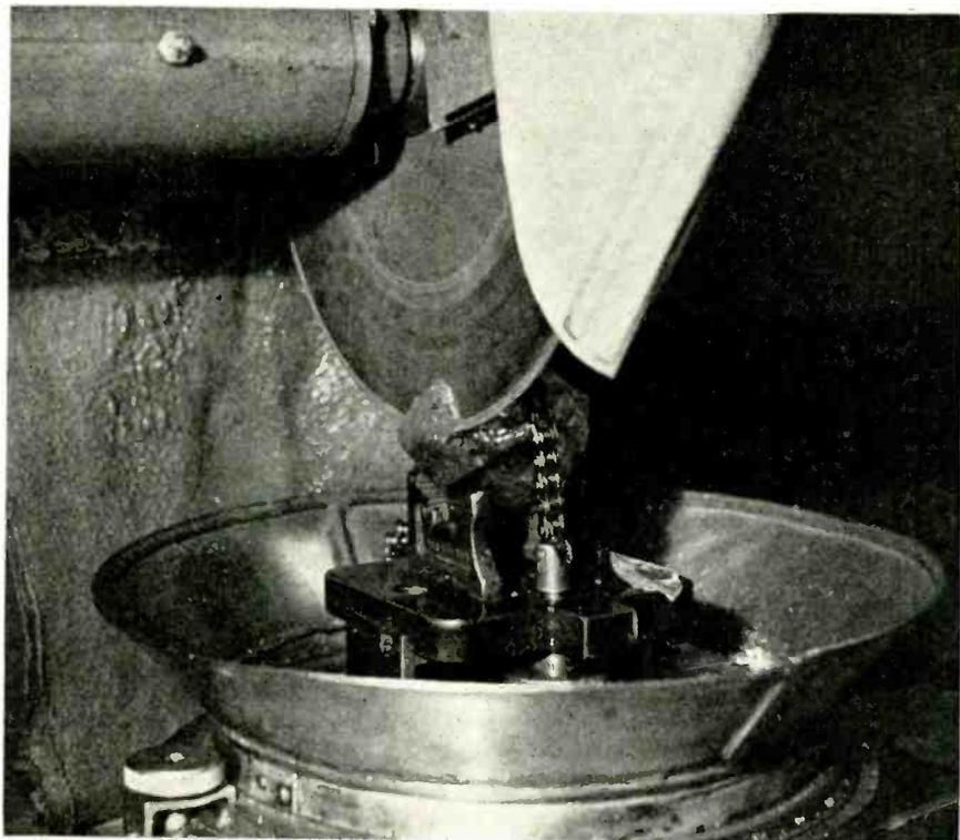
(Above). Close-up view of saw blade cutting end off raw crystal
