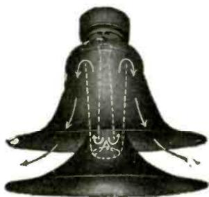
*Left*—RADIAL HORN SPEAKER; a 3½' re-entrant type horn. Projects sound over 360° area. Storm-proof. Made of RACON Acoustic Material to prevent resonant effects.
