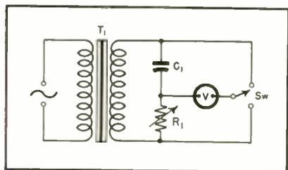
Fig. 1. Simple comparison method of measuring reactance
