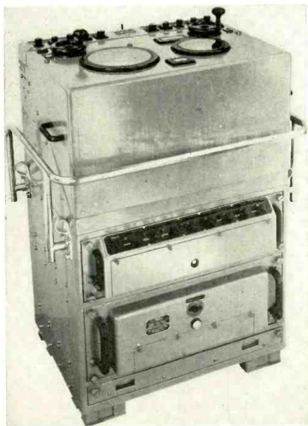
Above—View of top of precision radar repeater. Enlarged screen images shown at sides
