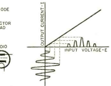
Screen grid and pentode tubes have been used to a limited extent as biased grid or plate circuit detectors. They have better sensitivity than triodes, but due to the extremely high output impedance, it is extremely difficult to realize much gain.
