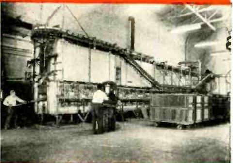
The largest sheets of mica ceramic insulation available (19 1/4" x 29 3/4") made only by Electronic Mechanics, are produced in this firing kiln followed by 12 to 36 hour annealing in the Lehr. This removes all internal stresses and strains in the sheets assuring great physical stability.
