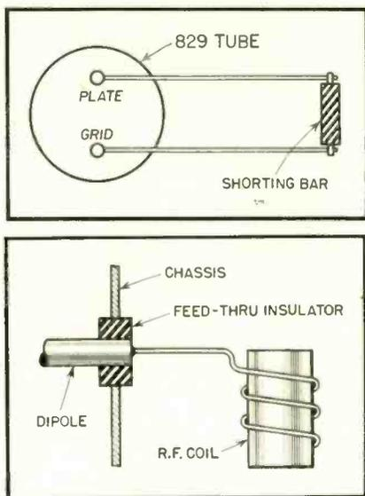
Fig. 4. Typical design applications of aniline laminates: shorting bar and feed-thru insulator
