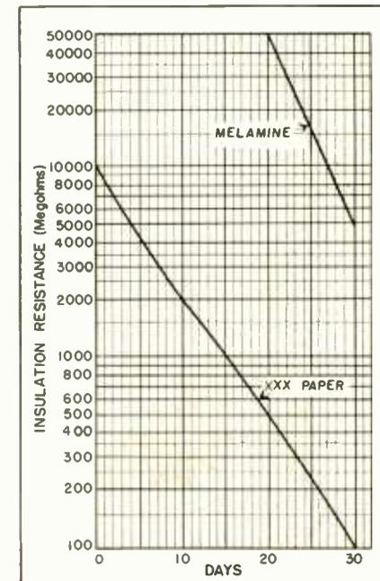
Fig. 2. Insulation resistance vs. time at 40° C. and 90% R.H.
