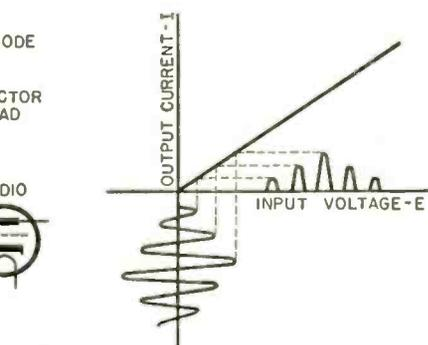
Screen grid and pentode tubes have been used to a limited extent as biased grid or plate circuit detectors. They have better sensitivity than triodes, but due to the extremely high output impedance, it is extremely difficult to realize much gain.
