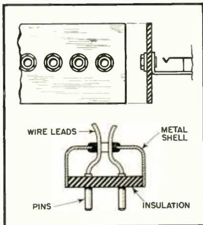
Fig. 1. Typical design uses of melamine laminates. Telephone jack panel board (above), and plug insulation
