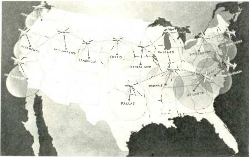
Airborne television and FM broadcasting system. This system, developed jointly by Westinghouse Electric Company and The Glenn L. Martin Company, proposes to beam (solid lines) programs originating in ground studios to planes for broadcast. Similarly beamed plane-to-plane connections (dotted lines) would form a nationwide network.
