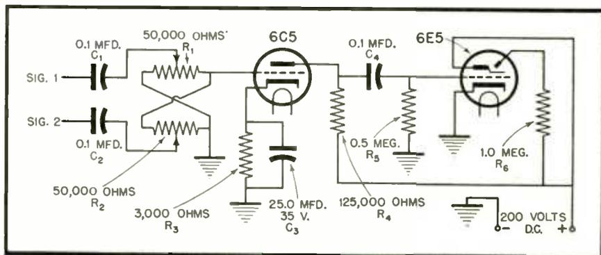
Fig. 3. Schematic of a sensitive indicator for synchronizing frequencies
