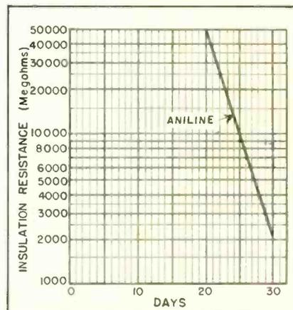
Fig. 5. Insulation resistance vs. time curve for aniline laminates
