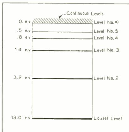
Fig. 3. Energy diagram of hydrogen atom
