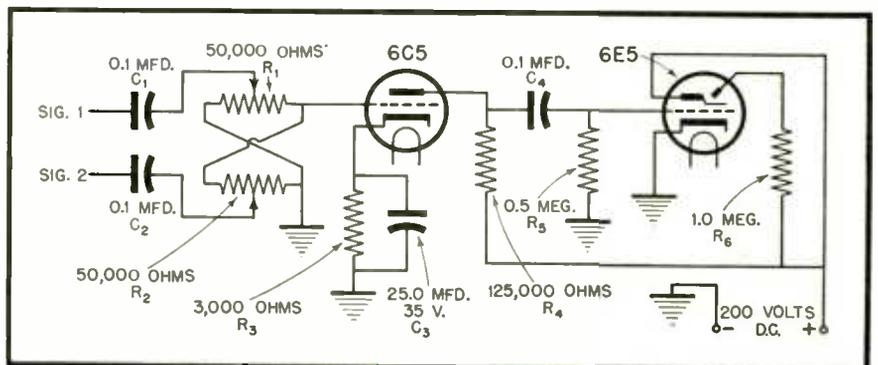
Fig. 3. Schematic of a sensitive indicator for synchronizing frequencies
