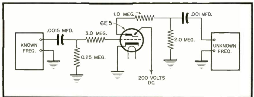
Fig. 2. Schematic of simple indicator for matching frequencies
