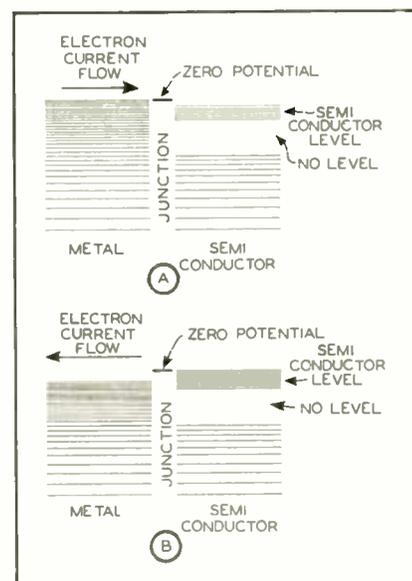
Fig. 5. Energy level diagrams of two types of rectifying junctions
