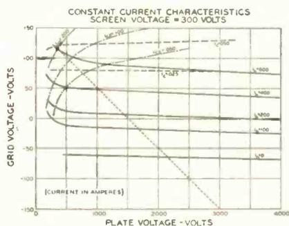
4-125A constant current characteristics. The operating line (short dashes) illustrates a 3000-volt, 500 watt input, 75 percent efficiency operating condition
