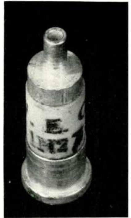
Fig. 2. The type 1N21-B crystal, a typical example of modern crystal rectifier construction
