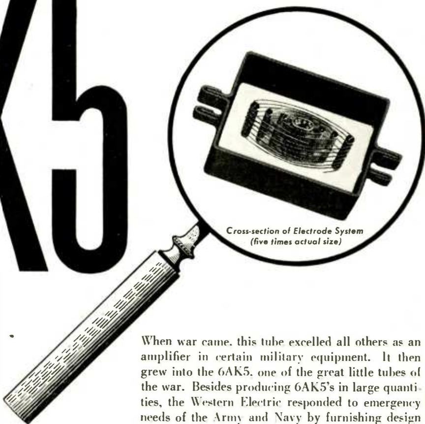
Cross-section of Electrode System
