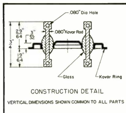
Fig. 4. Multiple conductor glass-to-metal terminal.
