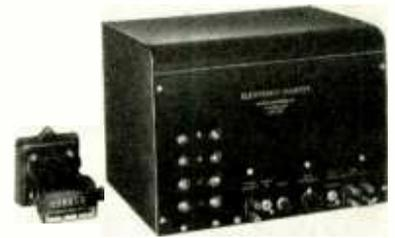
volved in the application of the two-decade electronic counter, it may be used alone, at counting rates up to 20,000 per second.
