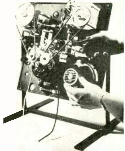
capable of making recordings on a moving steel wire and reproducing them immediately. It accomplishes this by producing small magnets along the moving wire according to the frequency and intensity of the audio signal, and converting the "peaks" and "valleys" of the moving magnetic field thus produced into sound by suitable electrical and mechanical means.
