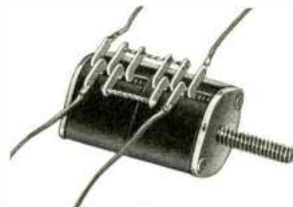
This new item is actually a double unit of Bradley's Model CX-4D4-F23, recently redesigned to handle much greater capacity than the original version. The single unit is now rated at 6 volts a.c. and 50 milliamperes d.c. continuous. It mounts on a single screw, is fully enclosed and completely sealed with a special plastic compound. Pre-soldered lead wires prevent overheating during assembly.
