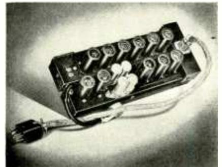
and a half-power bandwidth of 9.0 mc. An external gain control is easily provided. Unless otherwise specified, a standard 500 ohm input impedance is supplied. The output stages are cathode followers designed to operate into impedances of 75 to 100 ohms with voltages ranging from 0.5 to 2.0 volts, negative or positive.
