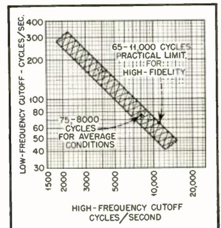
Fig. 6. Low and high frequency cutoff graph for tonal balance showing the comparative values both for average conditions and for high fidelity.
