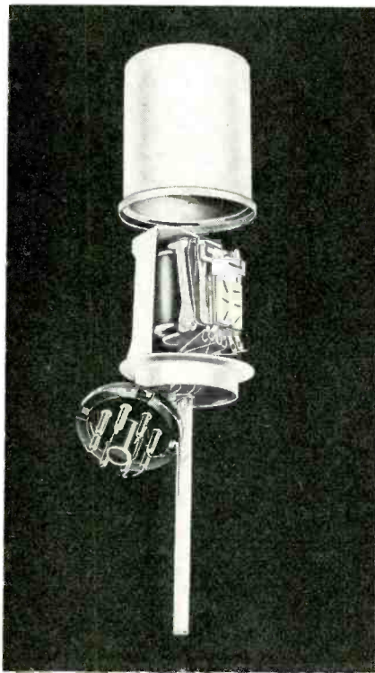
Fig. 9. Sealed relay. Air is exhausted from housing, which is filled with dry nitrogen.
