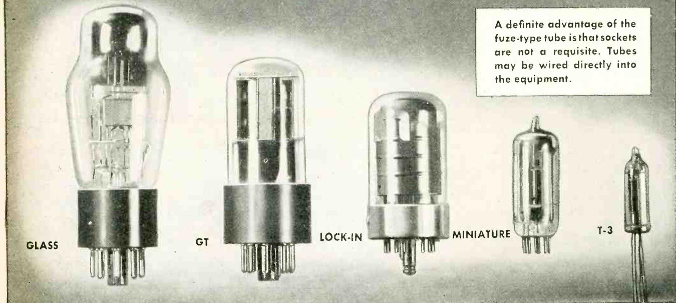
A definite advantage of the fuze-type tube is that sockets are not a requisite. Tubes may be wired directly into the equipment.
