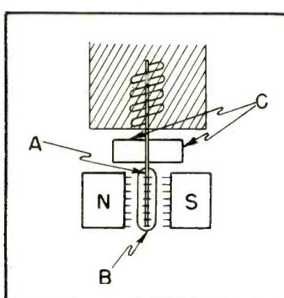
Fig. 1. Schematic view of pickup generating system
