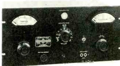
measurements on broadcast transmitters, the distortion meter operates from the high-impedance output circuit of the Type 1931-A modulation monitor. A continuous frequency range of 50 to 15,000 cycles, fundamental, is covered by a single dial and push-button multiplier. Distortion and noise components up to 45,000 cycles are included in the measurement. The direct-reading distortion meter provides full-
