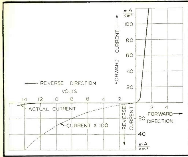
Fig. 3. D-c voltage-current characteristic for selenium rectifier plate. Reverse characteristic shown to 2 scales
