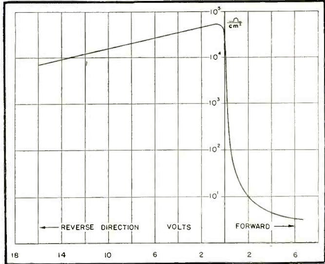
Fig. 4. Typical static resistance-voltage curve of selenium rectifier plate having an effective surface area of 1 sq. cm.
