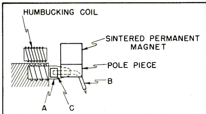
Fig. 2. Pickup side elevation, showing how stylus shank is bent
