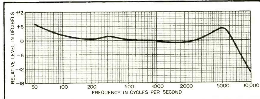
Fig. 4. Frequency response of pickup with damping applied
