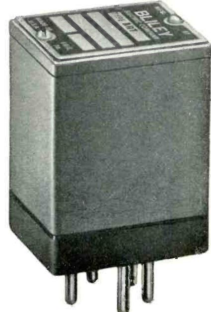
A built-in heater operating on 6.3 volts at 1 ampere provides temperature control within  $\pm 2^\circ\text{C}$ . This permits an over-all frequency tolerance of  $\pm .005\%$  or better including variations due to temperature change as well as tolerances required for crystal production.
