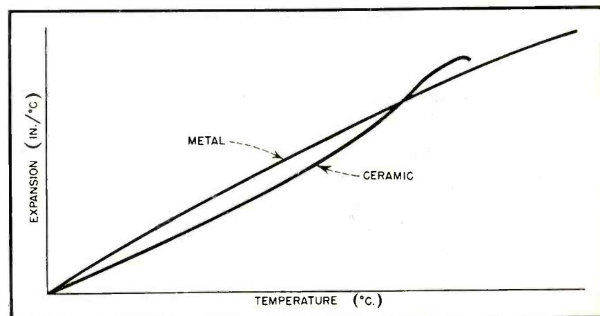
Fig. 3. Temperature-expansion chart of a typical metal-ceramic seal. Note the non-linearity of the ceramic material's expansion
