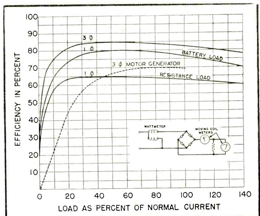
Fig. 5. Comparison of selenium rectifier efficiency at full load voltage with average typical efficiency of motor-generator set with exciters
