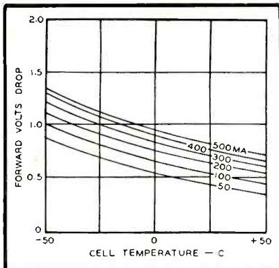
Fig. 6. Change in forward resistance vs. plate temperature
