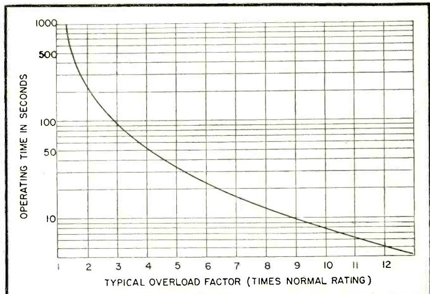
Fig. 9. Typical overload capacity curve
