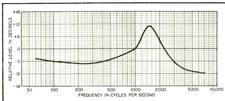
Fig. 3. Frequency characteristic of suspension shown in Figs. 1 and 2 without damping
