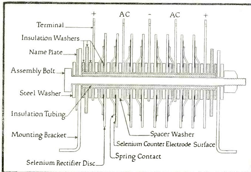
Fig. 2. Typical assembly of selenium rectifier
